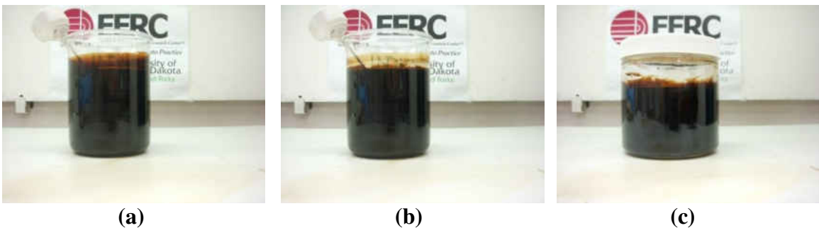
Figure 7-45. Lo-pour fuel oil – crude jatropha oil blend, mixed and held at 220°F. (a) immediately after five minutes of stirring, (b) 25 minutes after stirring, (c) three days after stirring.
