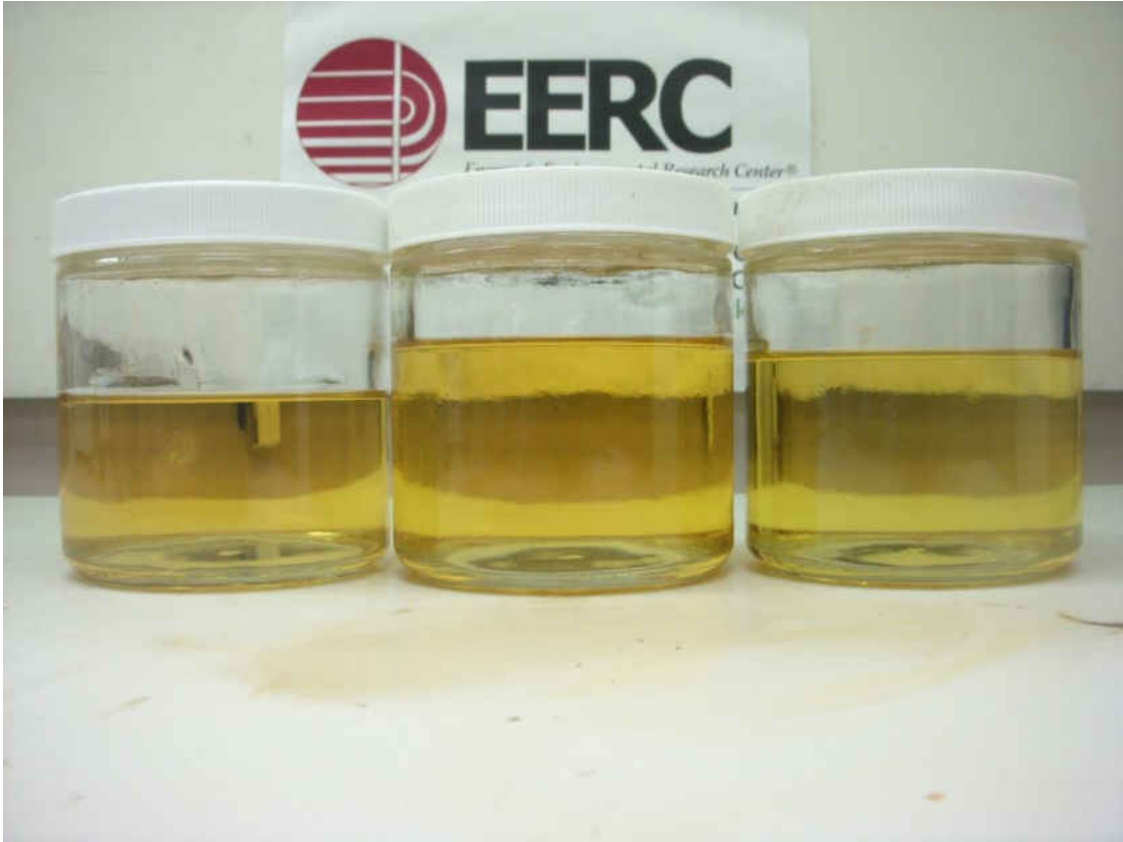
Figure 7-112. Crude jatropha oil – ultra-low sulfur diesel blend. In order from left to right, original blend temperatures were 75°F, 170°F, 220°F. All blends were photographed at 75°F.
