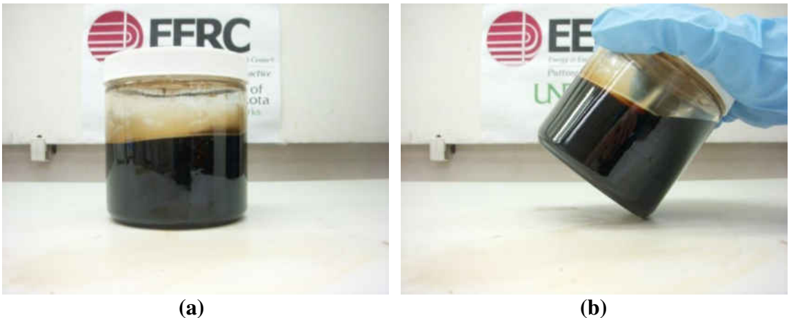
Figure 7-85. Lo-pour fuel oil – biodiesel blend, cooled from 220°F to 75°F. (a) shows the blend sitting flat, and (b) shows the blend tilted at an angle.
