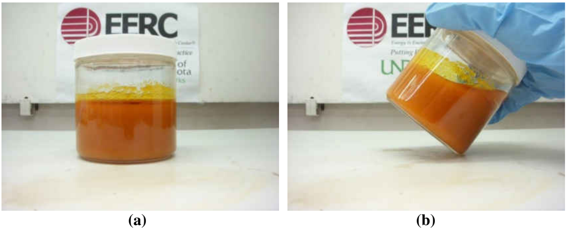
Figure 7-69. Crude palm oil – biocrude blend, cooled from 170°F to 75°F. (a) shows the blend sitting flat, and (b) shows the blend tilted at an angle.
