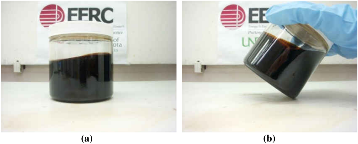
Figure 7-81. Hi-pour fuel oil – ultra-low sulfur diesel blend, cooled from 220°F to 75°F. (a) shows the blend sitting flat, and (b) shows the blend tilted at an angle.
