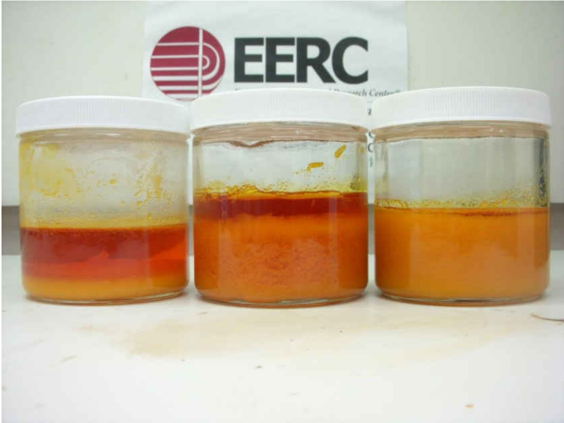
Figure 7-106. Crude palm oil – crude jatropha oil blend. In order from left to right, original blend temperatures were 75°F, 170°F, 220°F. All blends were photographed at 75°F.
