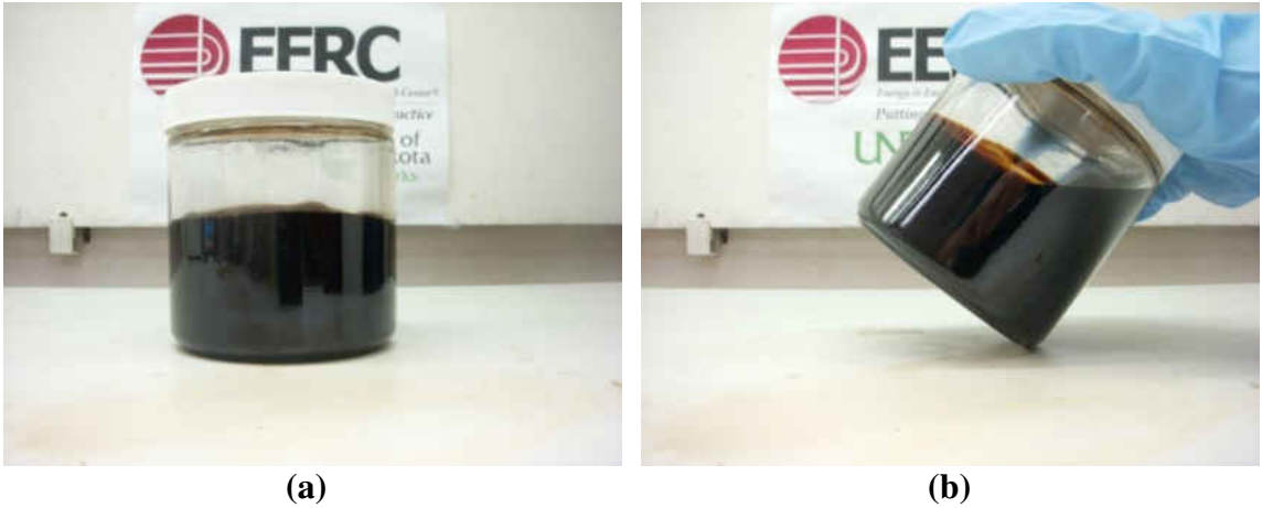
Figure 7-86. Lo-pour fuel oil – ultra-low sulfur diesel blend, cooled from 220°F to 75°F. (a) shows the blend sitting flat, and (b) shows the blend tilted at an angle.
