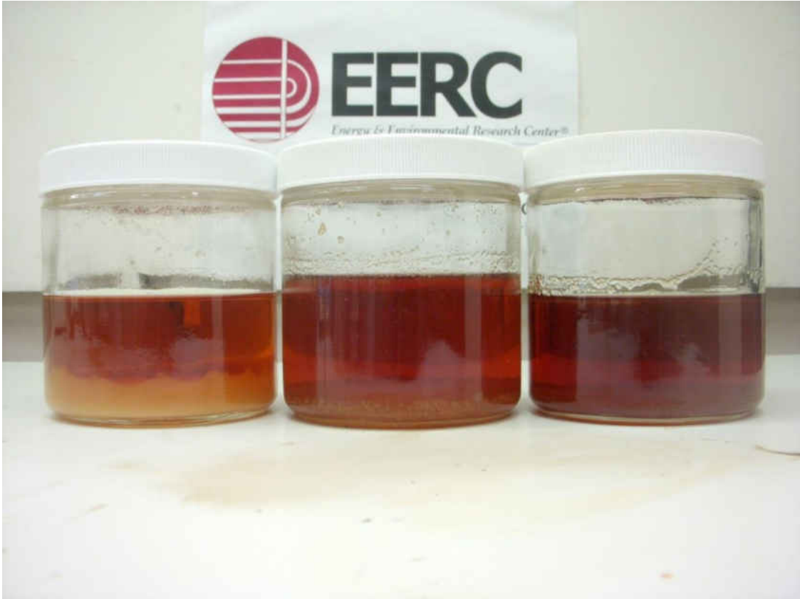
Figure 7-113. Biocrude – ultra-low sulfur diesel blend. In order from left to right, original blend temperatures were 75°F, 170°F, 220°F. All blends were photographed at 75°F.
