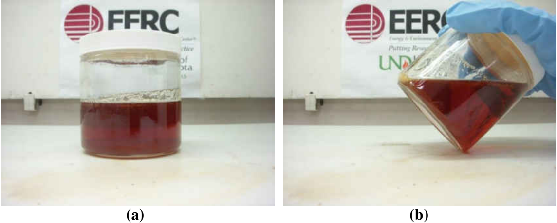
Figure 7-94. Biocrude – ultra-low sulfur diesel blend, cooled from 220°F to 75°F. (a) shows the blend sitting flat, and (b) shows the blend tilted at an angle.
