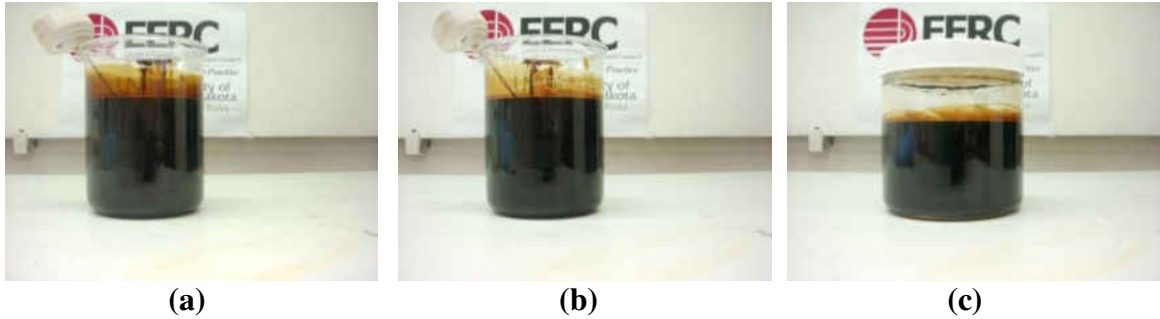
Figure 7-23. Hi-pour fuel oil – biodiesel blend, mixed and held at 170°F. (a) immediately after five minutes of stirring, (b) 25 minutes after stirring, (c) two days after stirring.
