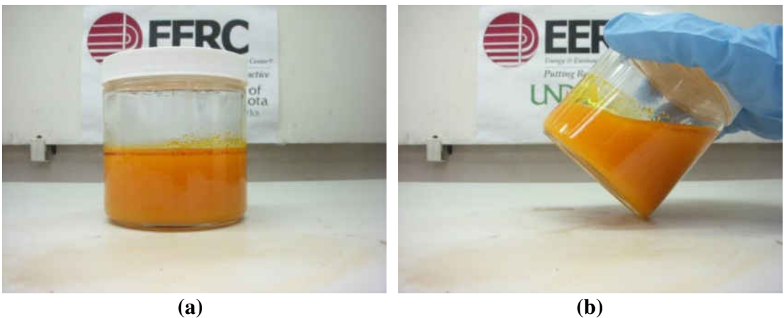
Figure 7-87. Crude palm oil – crude jatropha oil blend, cooled from 220°F to 75°F. (a) shows the blend sitting flat, and (b) shows the blend tilted at an angle.
