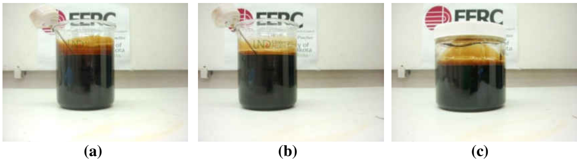
Figure 7-24. Hi-pour fuel oil – ultra-low sulfur diesel blend, mixed and held at 170°F. (a) immediately after five minutes of stirring, (b) 25 minutes after stirring, (c) two days after stirring.
