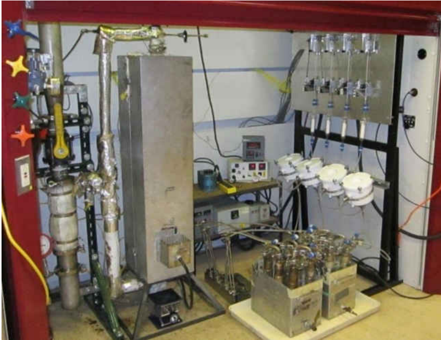
Figure 3-4. Laboratory-scale updraft gasifier and tar cracker.
