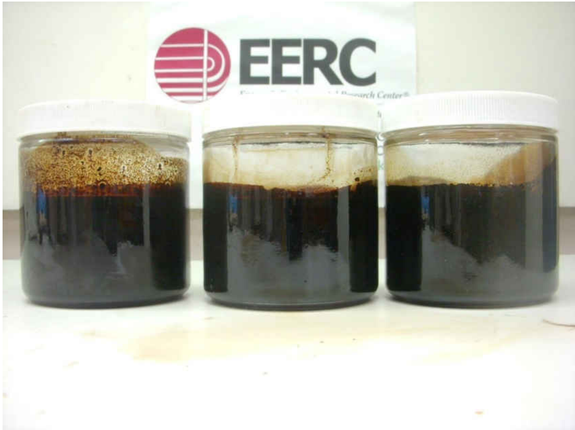
Figure 7-96. Hi-pour fuel oil – crude palm oil blend. In order from left to right, original blend temperatures were 75°F, 170°F, 220°F. All blends have been photographed at 75°F.
