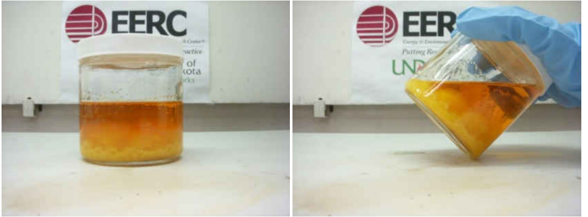
(a) (b) Figure 7-90. Crude palm oil – ultra-low sulfur diesel blend, cooled from 220°F to 75°F. (a) shows the blend sitting flat, and (b) shows the blend tilted at an angle.
