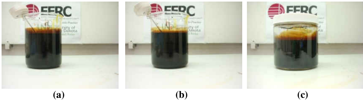
Figure 7-20. Hi-pour fuel oil – crude palm oil blend, mixed and held at 170°F. (a) immediately after five minutes of stirring, (b) 25 minutes after stirring, (c) two days after stirring.
