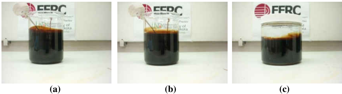
Figure 7-22. Hi-pour fuel oil – biocrude blend, mixed and held at 170°F. (a) immediately after five minutes of stirring, (b) 25 minutes after stirring, (c) two days after stirring.
