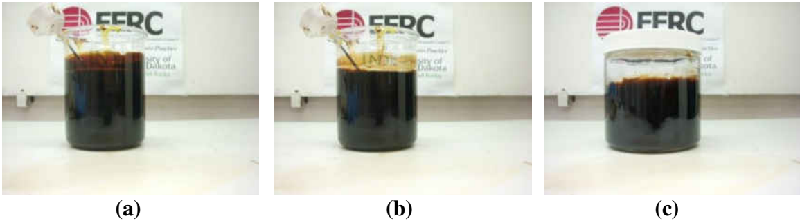
Figure 7-44. Lo-pour fuel oil – crude palm oil blend, mixed and held at 220°F. (a) immediately after five minutes of stirring, (b) 25 minutes after stirring, (c) three days after stirring.
