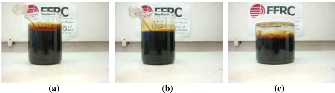
Figure 7-43. Hi-pour fuel oil – ultra-low sulfur diesel blend, mixed and held at 220°F. (a) immediately after five minutes of stirring, (b) 25 minutes after stirring, (c) three days after stirring.
