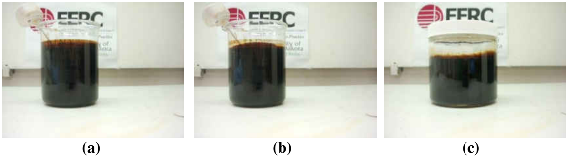
Figure 7-27. Lo-pour fuel oil – biocrude blend, mixed and held at 170°F. (a) immediately after five minutes of stirring, (b) 25 minutes after stirring, (c) four days after stirring.
