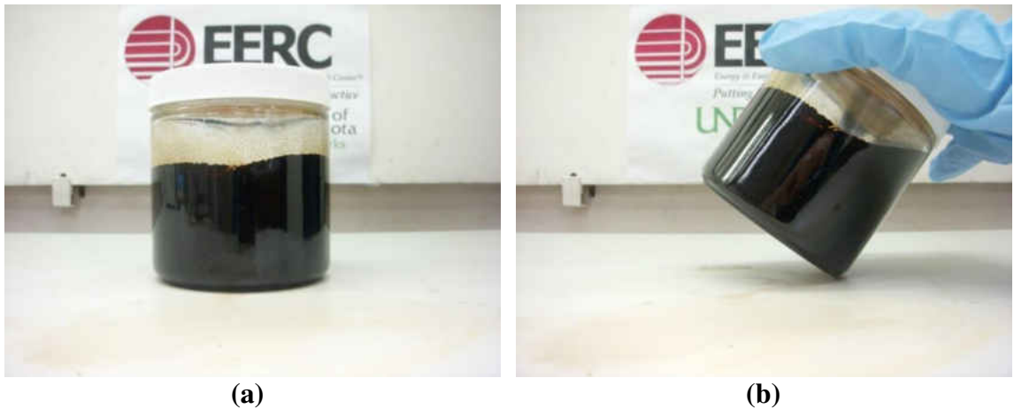
Figure 7-77. Hi-pour fuel oil – crude palm oil blend, cooled from 220°F to 75°F. (a) shows the blend sitting flat, and (b) shows the blend tilted at an angle.
