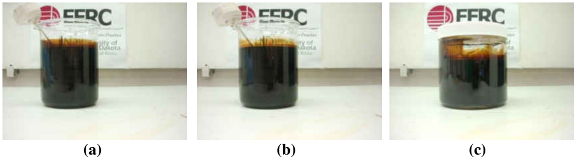
Figure 7-21. Hi-pour fuel oil – crude jatropha oil blend, mixed and held at 170°F. (a) immediately after five minutes of stirring, (b) 25 minutes after stirring, (c) two days after stirring.
