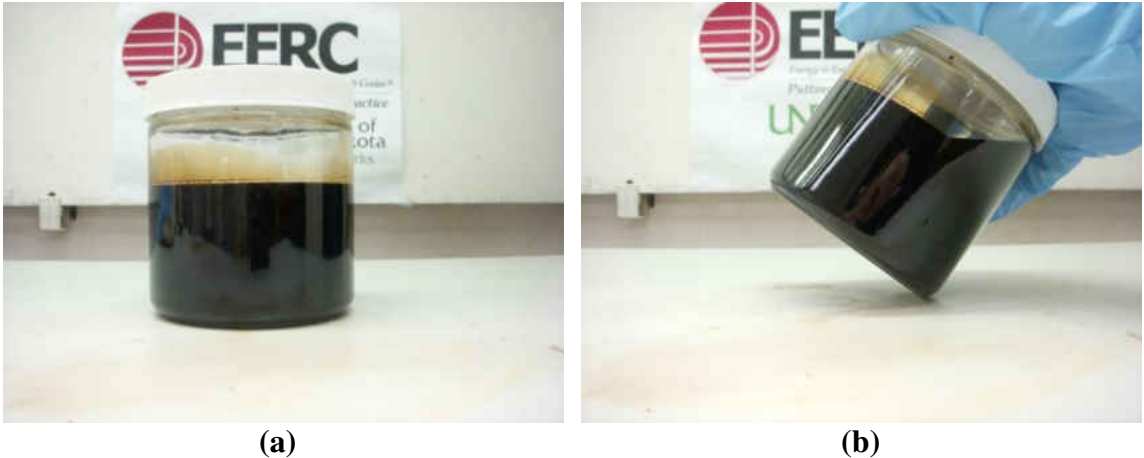
Figure 7-65. Lo-pour fuel oil – biocrude blend, cooled from 170°F to 75°F. (a) shows the blend sitting flat, and (b) shows the blend tilted at an angle.
