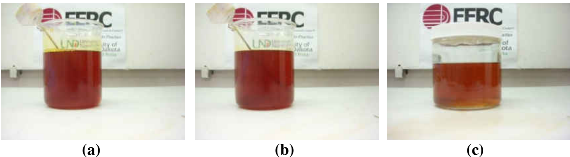
Figure 7-51. Crude palm oil – biodiesel blend, mixed and held at 220°F. (a) immediately after five minutes of stirring, (b) 25 minutes after stirring, (c) five days after stirring.
