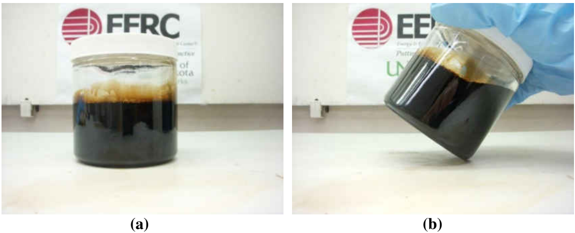
Figure 7-63. Lo-pour fuel oil – crude palm oil blend, cooled from 170°F to 75°F. (a) shows the blend sitting flat, and (b) shows the blend tilted at an angle.
