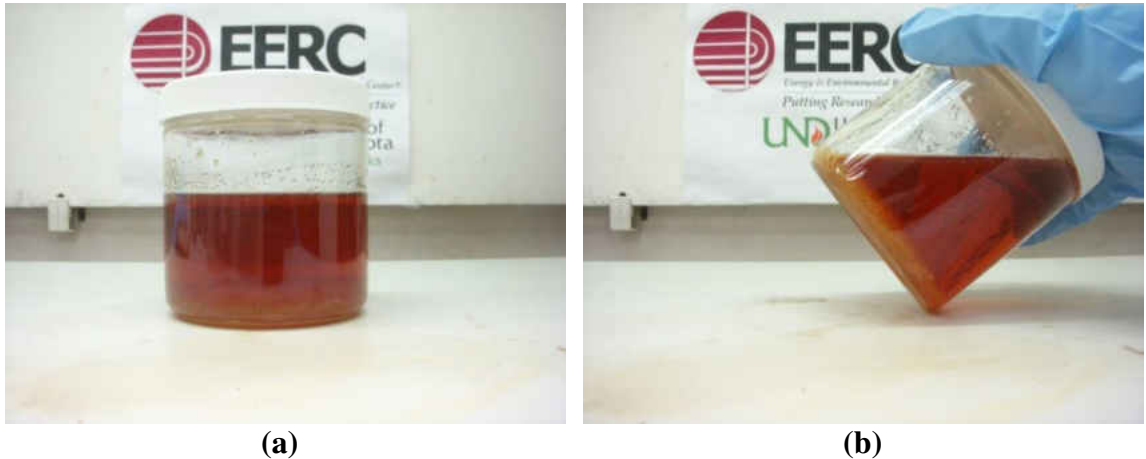
Figure 7-75. Biocrude – ultra-low sulfur diesel blend, cooled from 170°F to 75°F. (a) shows the blend sitting flat, and (b) shows the blend tilted at an angle.
