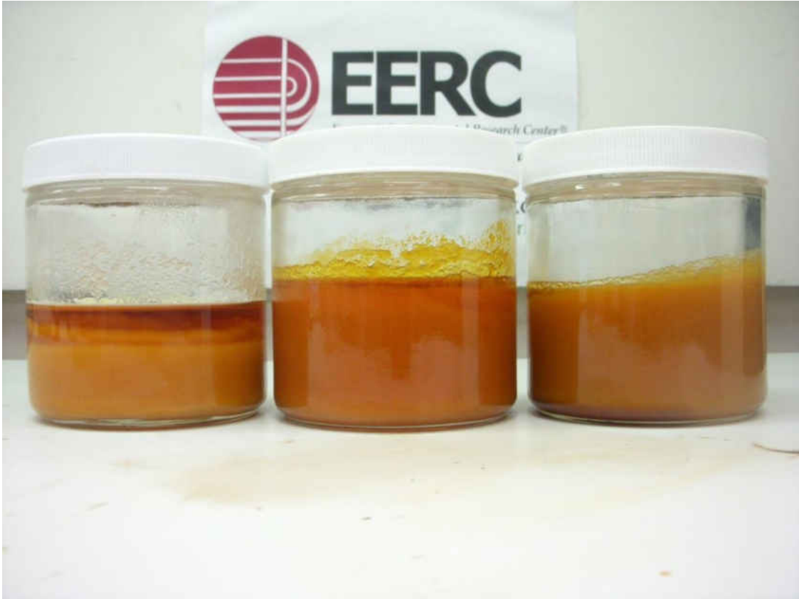
Figure 7-107. Crude palm oil – biocrude blend. In order from left to right, original blend temperatures were 75°F, 170°F, 220°F. All blends were photographed at 75°F.
