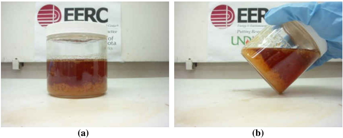
Figure 7-72. Crude jatropha oil – biocrude blend, cooled from 170°F to 75°F. (a) shows the blend sitting flat, and (b) shows the blend tilted at an angle.
