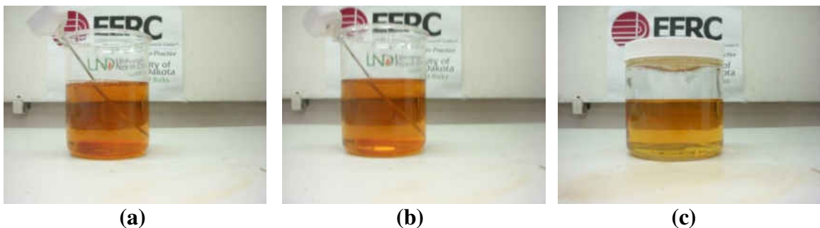
Figure 7-57. Biodiesel – ultra-low sulfur diesel blend, mixed and held at 220°F. (a) immediately after five minutes of stirring, (b) 25 minutes after stirring, (c) six days after stirring.
