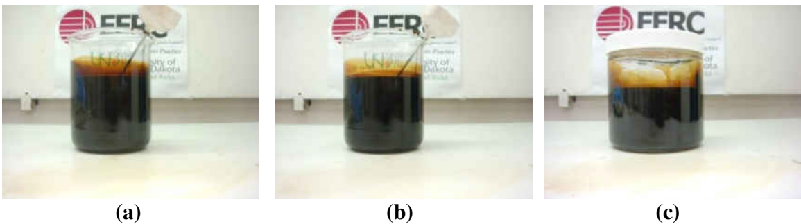
Figure 7-39. Hi-pour fuel oil – crude palm oil blend, mixed and held at 220°F. (a) immediately after five minutes of stirring, (b) 25 minutes after stirring, (c) three days after stirring.
