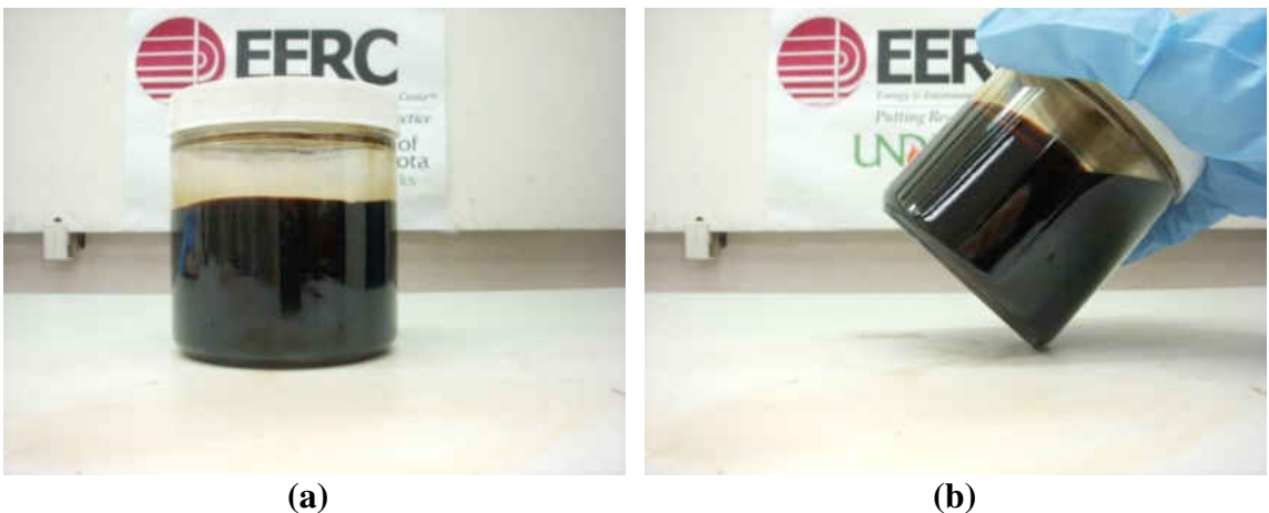
Figure 7-66. Lo-pour fuel oil – biodiesel blend, cooled from 170°F to 75°F. (a) shows the blend sitting flat, and (b) shows the blend tilted at an angle.
