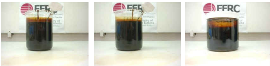
(a) (b) (c) Figure 7-40. Hi-pour fuel oil – crude jatropha oil blend, mixed and held at 220°F. (a) immediately after five minutes of stirring, (b) 25 minutes after stirring, (c) three days after stirring.
