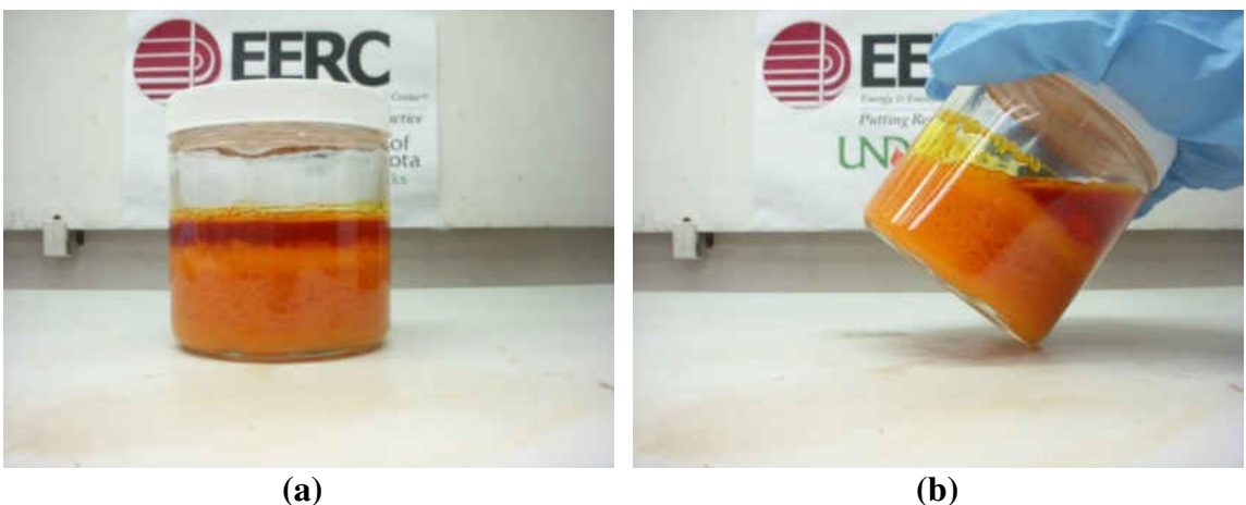
Figure 7-68. Crude palm oil – crude jatropha oil blend, cooled from 170°F to 75°F. (a) shows the blend sitting flat, and (b) shows the blend tilted at an angle.
