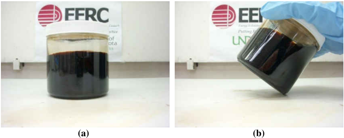
Figure 7-80. Hi-pour fuel oil – biodiesel blend, cooled from 220°F to 75°F. (a) shows the blend sitting flat, and (b) shows the blend tilted at an angle.
