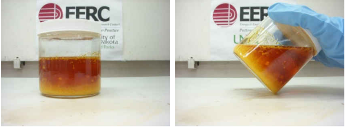
(a) (b) Figure 7-89. Crude palm oil – biodiesel blend, cooled from 220°F to 75°F. (a) shows the blend sitting flat, and (b) shows the blend tilted at an angle.
