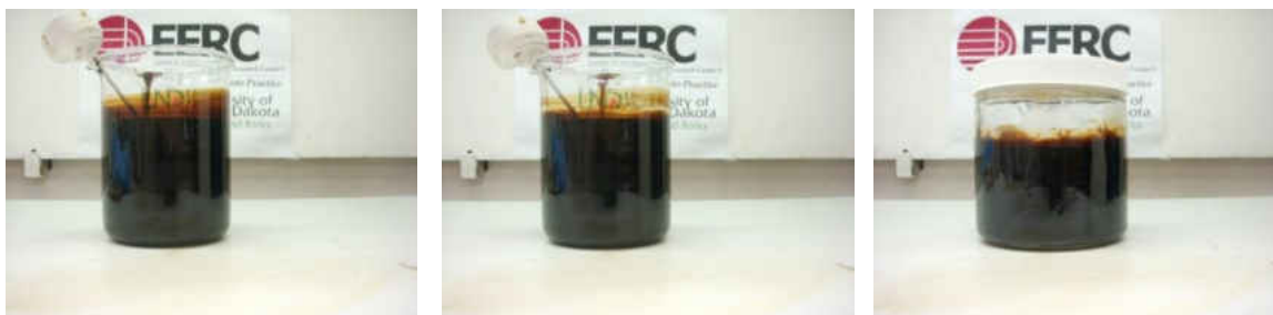
(a) (b) (c) Figure 7-41. Hi-pour fuel oil – biocrude blend, mixed and held at 220°F. (a) immediately after five minutes of stirring, (b) 25 minutes after stirring, (c) three days after stirring.
