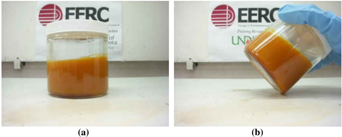
Figure 7-88. Crude palm oil – biocrude blend, cooled from 220°F to 75°F. (a) shows the blend sitting flat, and (b) shows the blend tilted at an angle.
