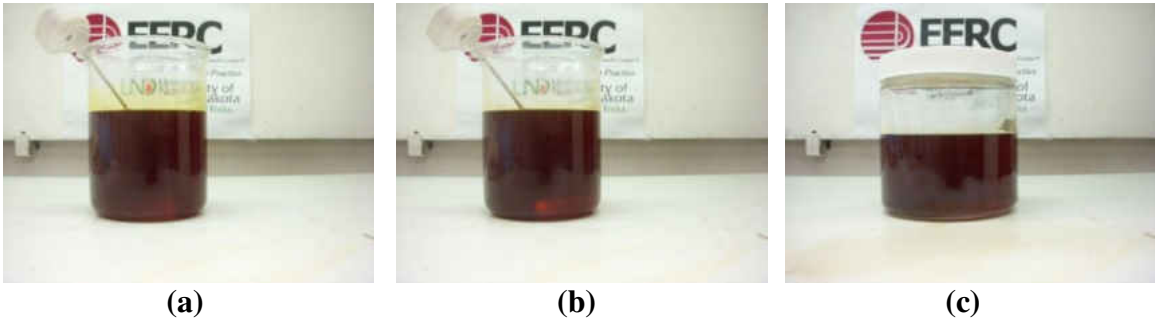
Figure 7-50. Crude palm oil – biocrude blend, mixed and held at 220°F. (a) immediately after five minutes of stirring, (b) 25 minutes after stirring, (c) five days after stirring.
