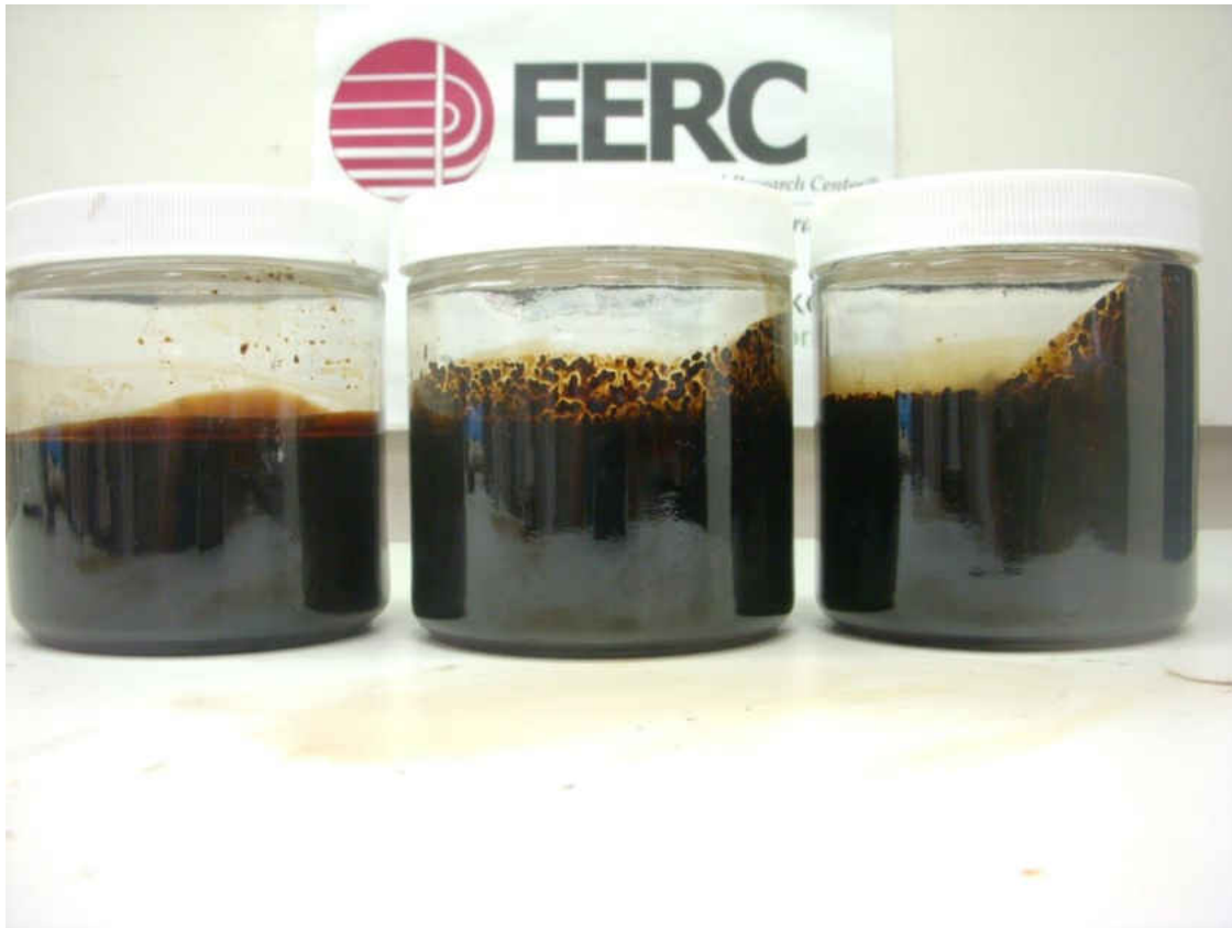
Figure 7-101. Lo-pour fuel oil – crude palm oil blend. In order from left to right, original blend temperatures were 75°F, 170°F, 220°F. All blends were photographed at 75°F.
