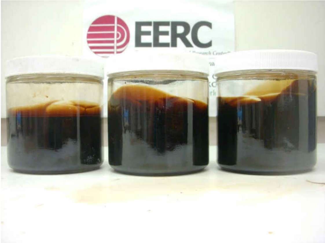
Figure 7-100. Hi-pour fuel oil – ultra-low sulfur diesel blend. In order from left to right, original blend temperatures were 75°F, 170°F, 220°F. All blends were photographed at 75°F.
