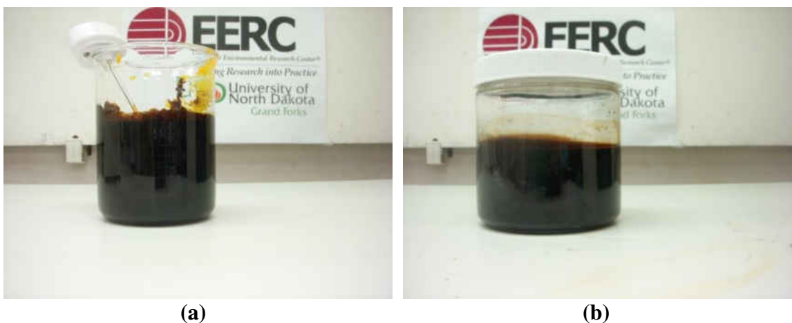
Figure 7-6. Lo-pour fuel oil – crude palm oil blend, mixed and held at 75°F. (a) immediately after attempted blending, (b) 492 days after attempted blending.
