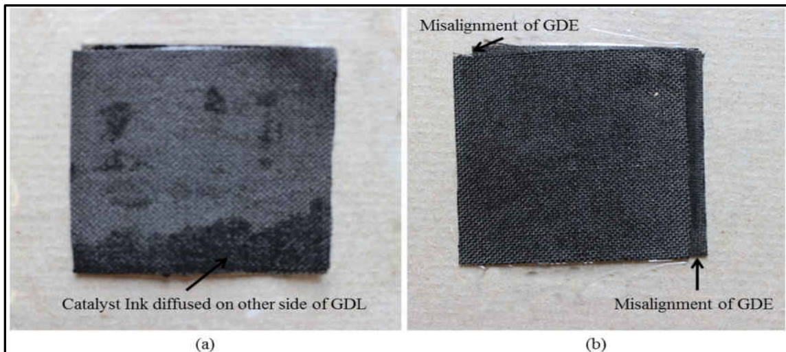
Figure 6-4 In-house fabricated MEA rejected for (a) catalyst ink diffused through the GDL to the other side (b) improper alignment of the GDEs around the electrolyte membrane
