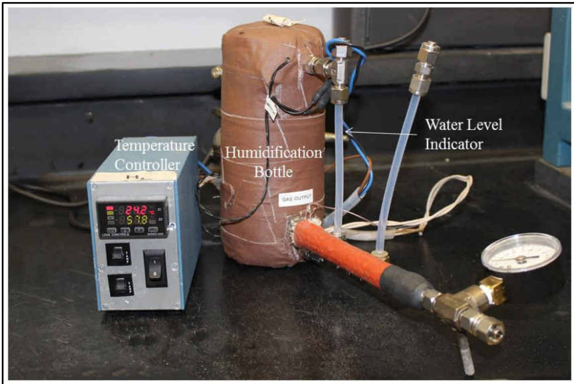
Figure 4-14 Humidification System used for reactants humidification
