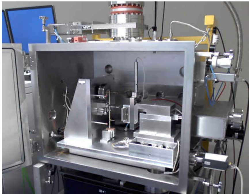
Figure 3.7. The NanoTest Xtreme nanoindenter (Micro Materials, UK) situated inside the vacuum chamber [6].
