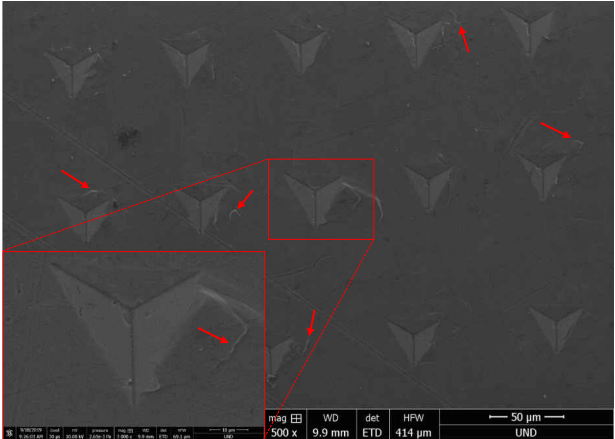
Figure 4.10. Scanning electron microscopy (SEM) image of Berkovich indentations made on pure Mg at 500x magnification and a close-up of a single indentation made at 3,000x magnification (inset). Red arrows point out microcracks near indentations.
