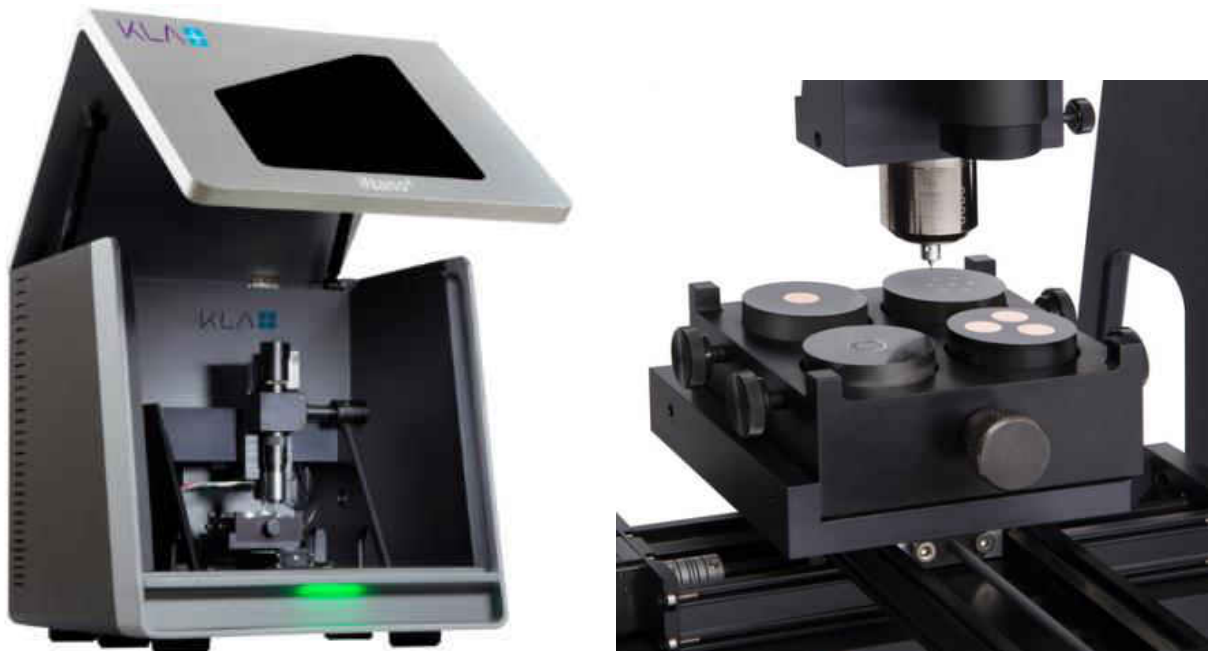
Figure 3.3. KLA-Tencor iNano nanoindenter (left) and indentation platform (right).
