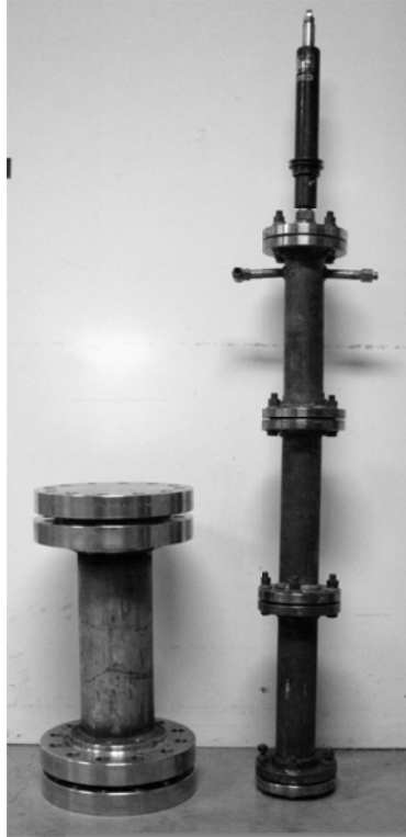
Figure 103. New CSTR vs. old PFR visual comparison.
