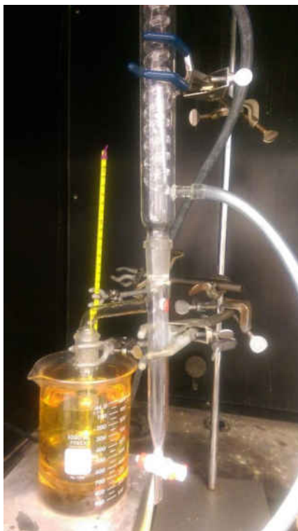
Figure 27: Reflux apparatus used in the synthesis of hydroxyl-polyimides, specifically in the conversion of hydroxyl-polyamic acid to hydroxyl-polyimide
