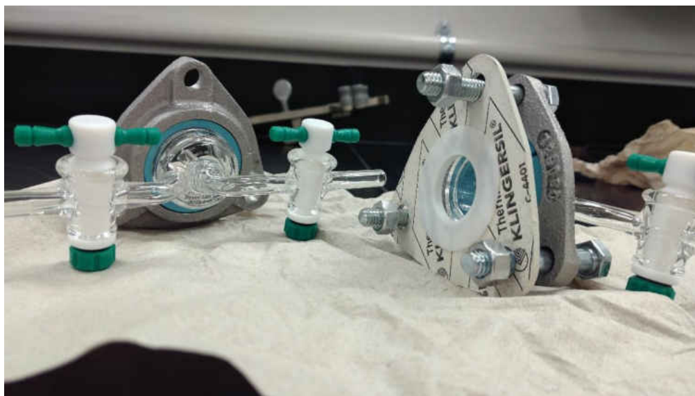
Figure 22: Open PTC 700 1" Test Cell for Vapor Phase Testing from Pesce Labs, Inc.
