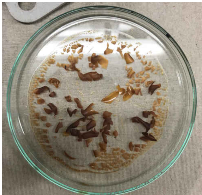
Figure 43. Resulting polyimide "membrane" synthesized from reactant ratio of 1:0.5 of diamine: dianhydride.
