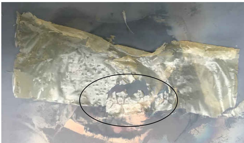
Figure 45. Image of the membrane fabricated using the recrystallized diamine with ODPA.
