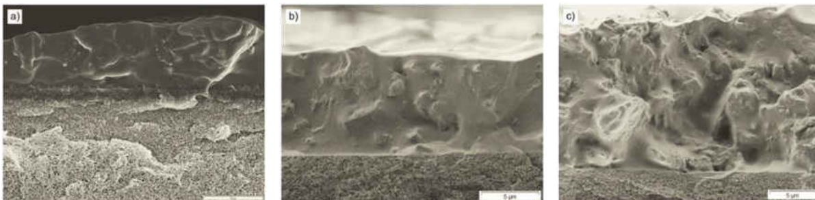
Figure 8: POMS membranes formed with AC loaded with (a) 10 wt.% (b) 20 wt.% (c) 40 wt.% showing the increase in inhomogeneity with increasing amounts of AC (89). Reprinted with permission from Wiley.
