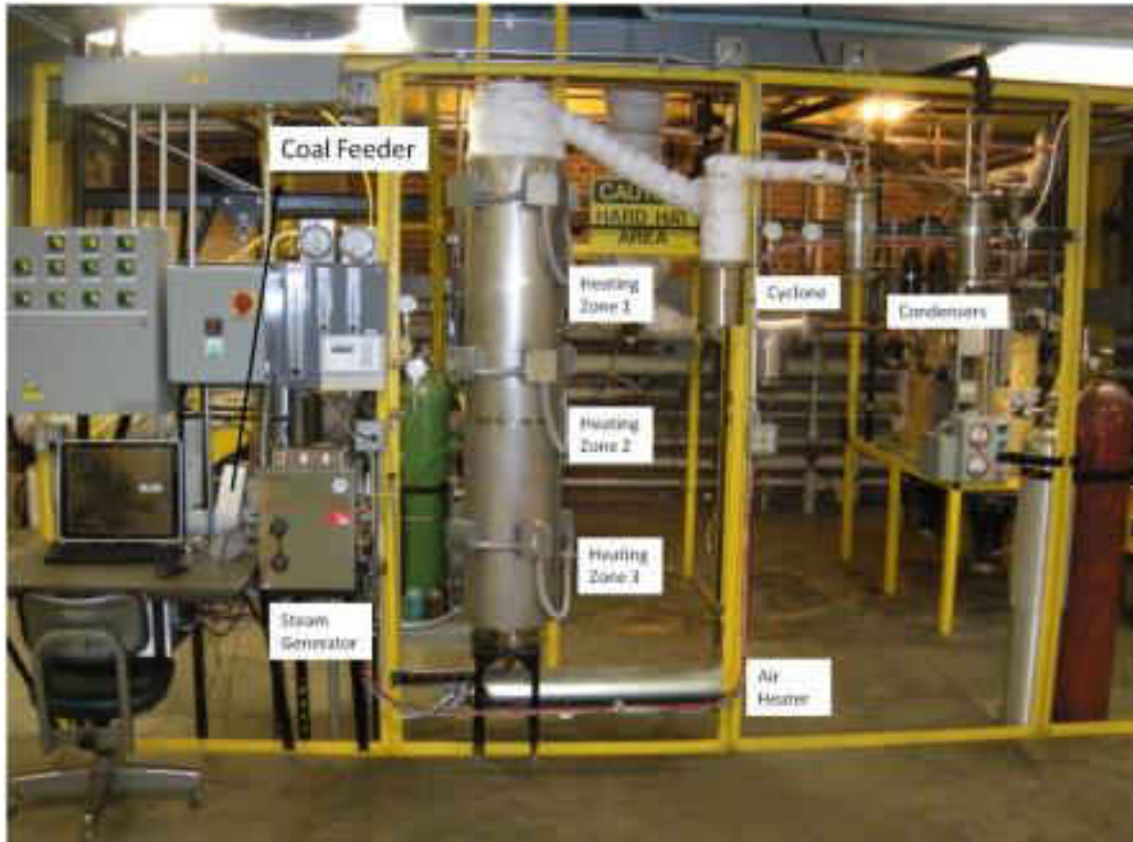
Figure 3-2: Original gasification design by Robert Mota[1].
