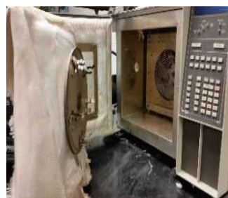
Figure IV-1: Small Batch Reactor used in Temperature Studies
