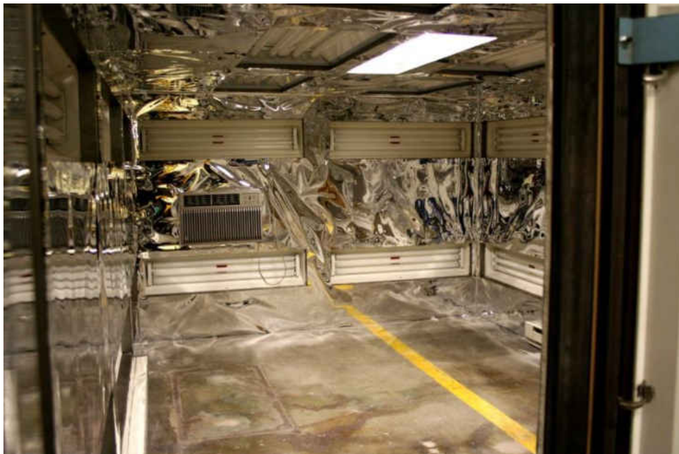
Figure 8. Inside of The University of North Dakota (UND) atmospheric chamber enclosure showing UV light fixtures, reflective mirror sheeting and air conditioning units.
