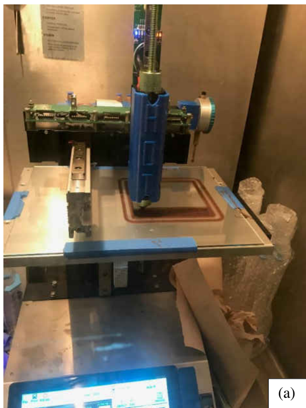
Figure 2.1: Schematics of, (a) a 3D printer printing PLA-50 wt% Lignin composition, and (b) a PLA-50 wt% Lignin 3D printed sample.
