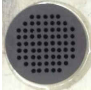
Fig. 3.1.1 Sintered ferrite sample with holes drilled.
