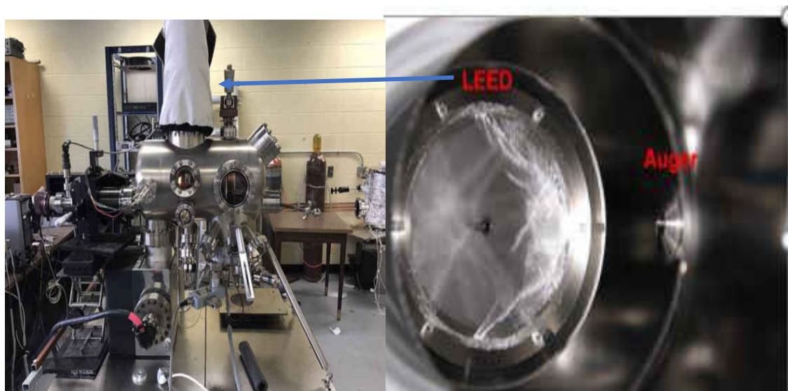
Figure 2.5 (a) UHV set up with LEED (b) LEED screen
