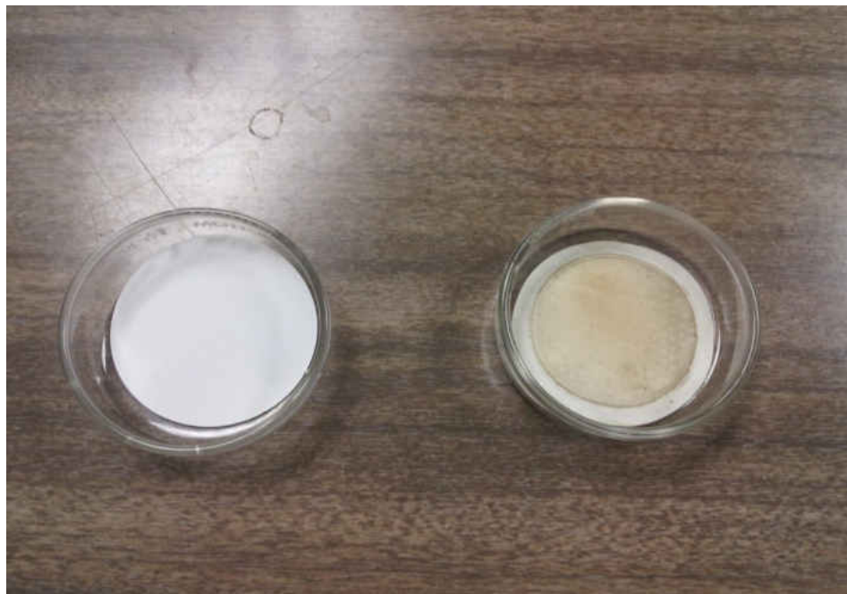
Figure 27: Before (left) and after (right) pervaporation image of polyamide composite membrane
