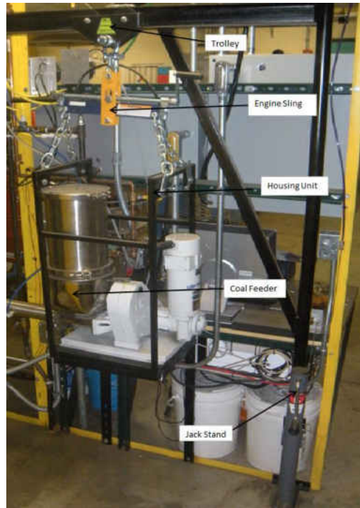
Figure 3: Coal feeding system
