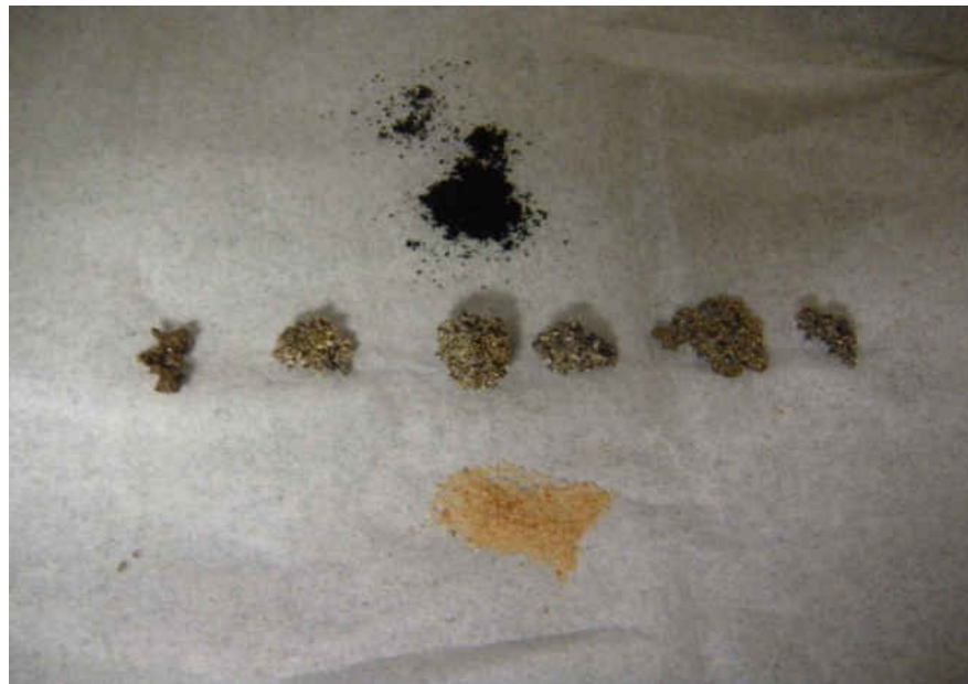
Figure 37: Agglomeration formation under combustion conditions.
