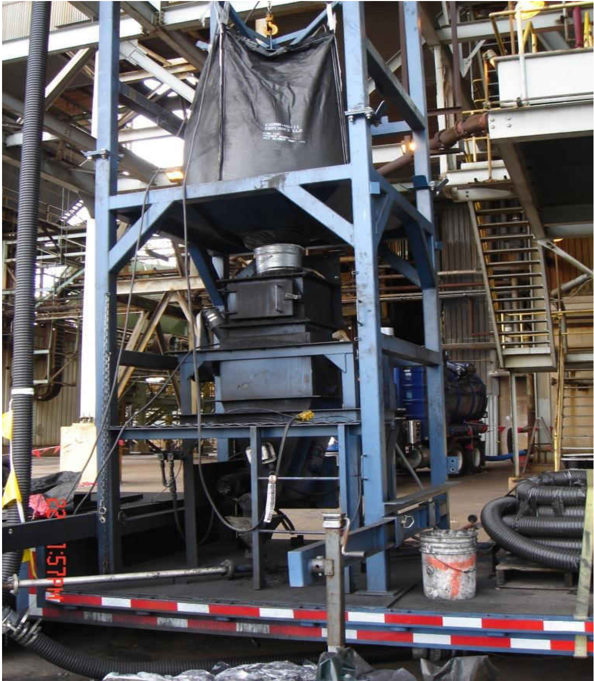
Figure 24: Close-up view of bulk/sorbent bag handling system and discharge hose
