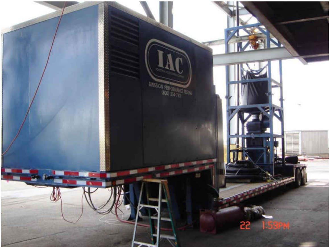
Figure 23: Sorbent injection trailer with blower and compressor housing; bulk bag lifter assembled, and the bulk bag in place.
