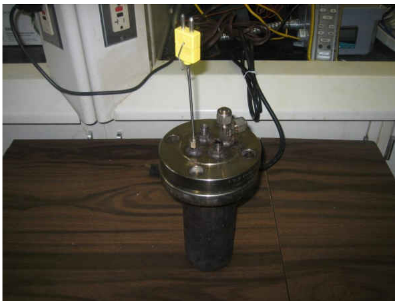
Figure A.1: Photograph of the Coking Reactor Vessel
