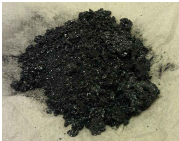
Figure A.3: Photograph of Green Coke
