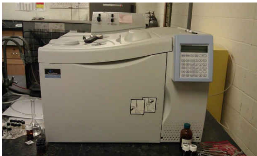
Figure 16: Photograph of the Perkin Elmer Clarus 480 Gas Chromatograph SimDist
