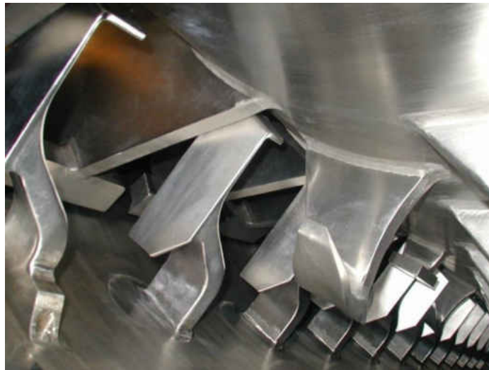
Figure 7: Photograph of the blades inside of a Continuous Coking Furnace [20]
