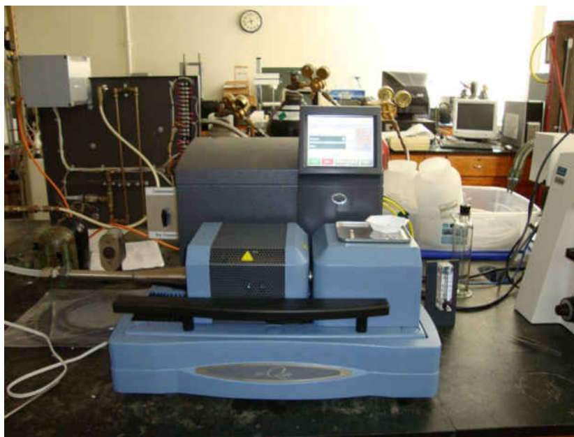
Figure 15: Photograph of the TA Instruments SDT Q600 TGA
