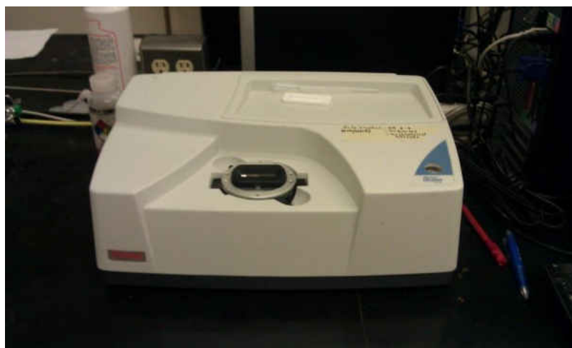
Figure 17: Photograph of the Thermo Scientific Nicolet IR 200 FT-IR
