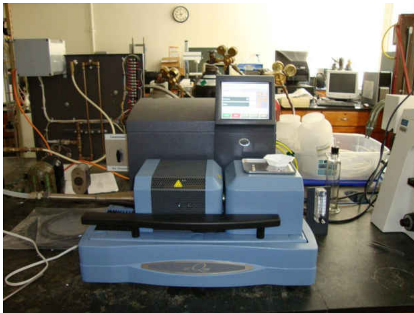
Figure 10: Photograph of the TA Instruments SDT Q600 TGA
