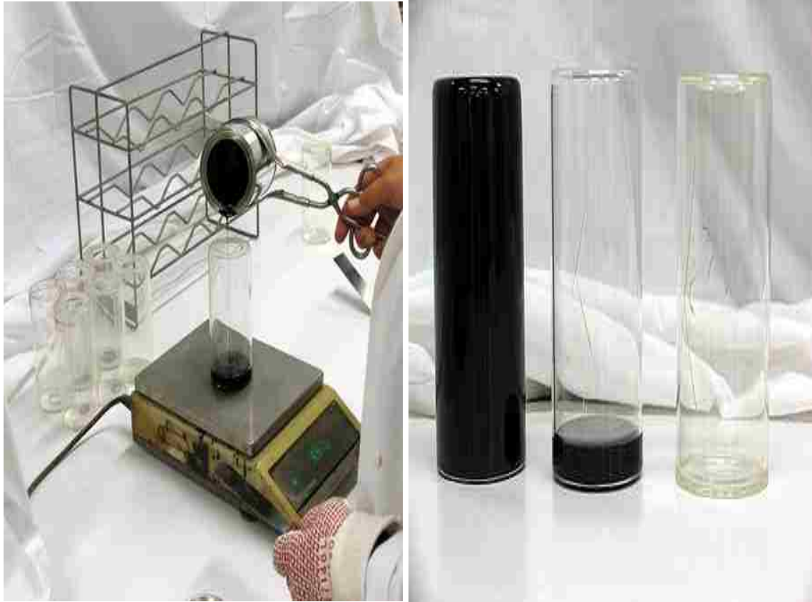
Figure 3.1: Sample preparation for RTFO test [39].
