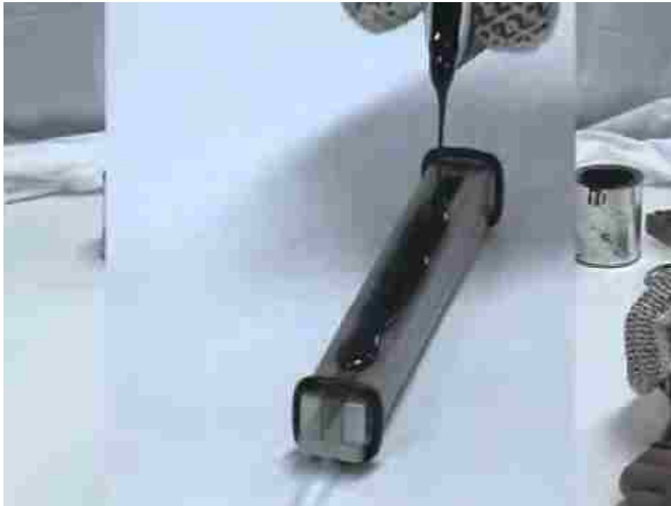
Figure 3.5: Preparation of BBR beams [46].
