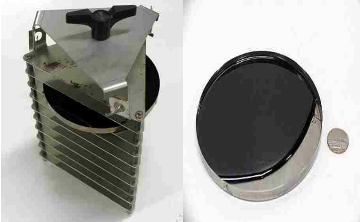
Figure 3.2: Sample preparation for PAV tests [42].
