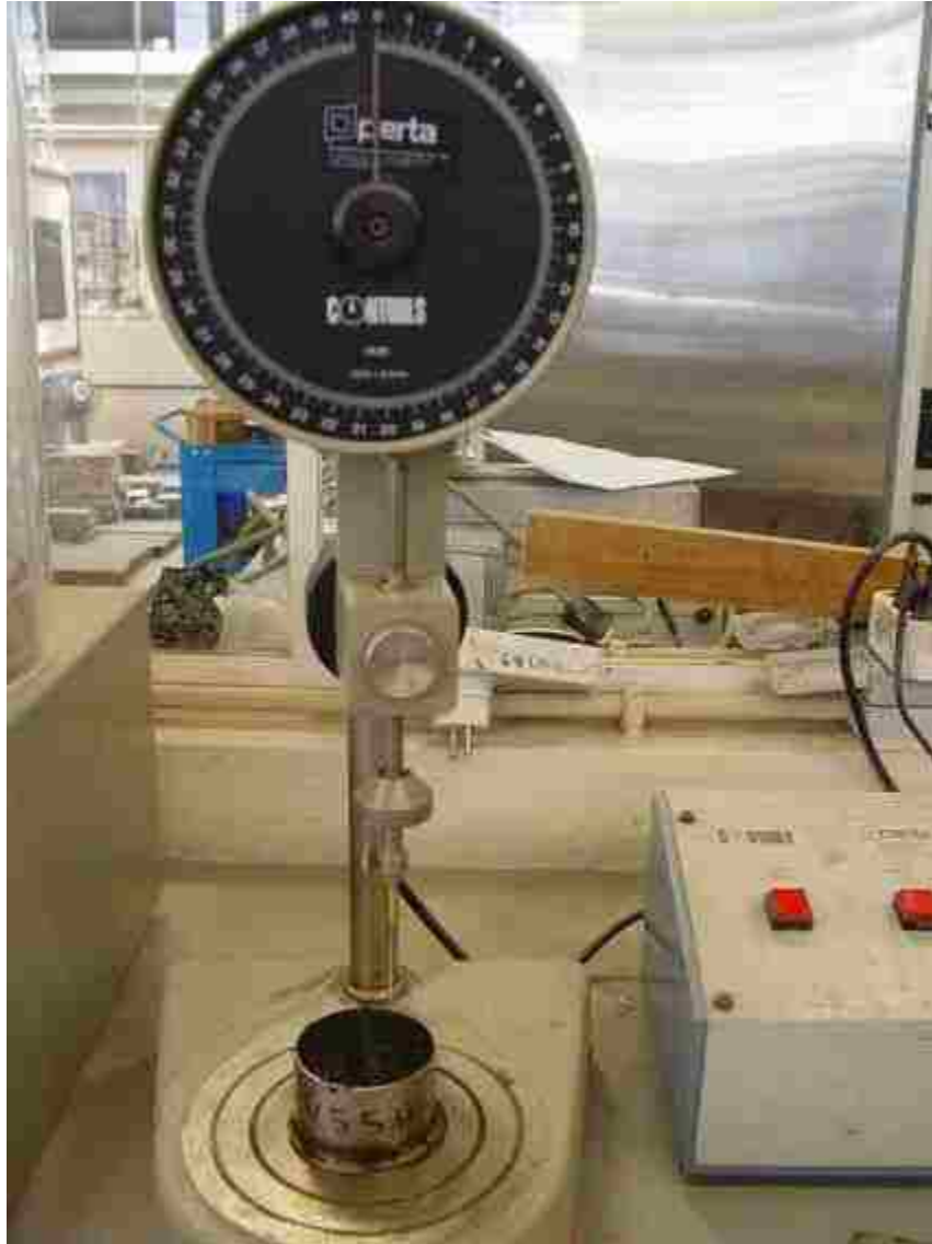
Figure 2.5: Penetration test equipment [35].
