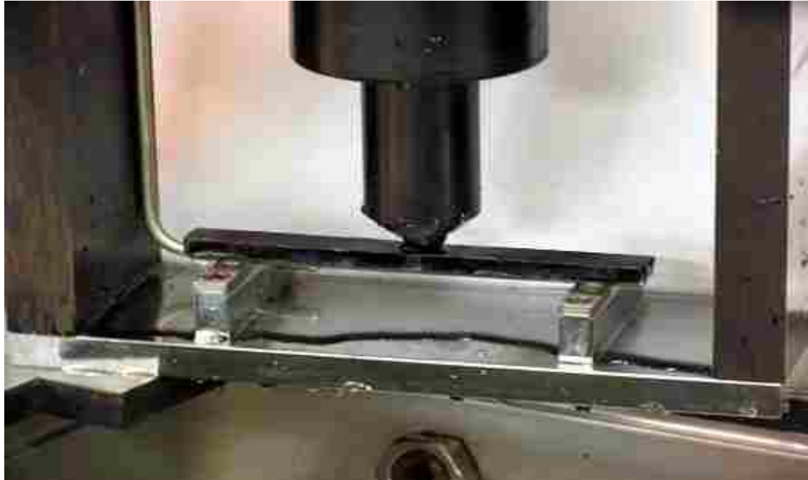
Figure 3.6: BBR beam ready to be tested [46].
