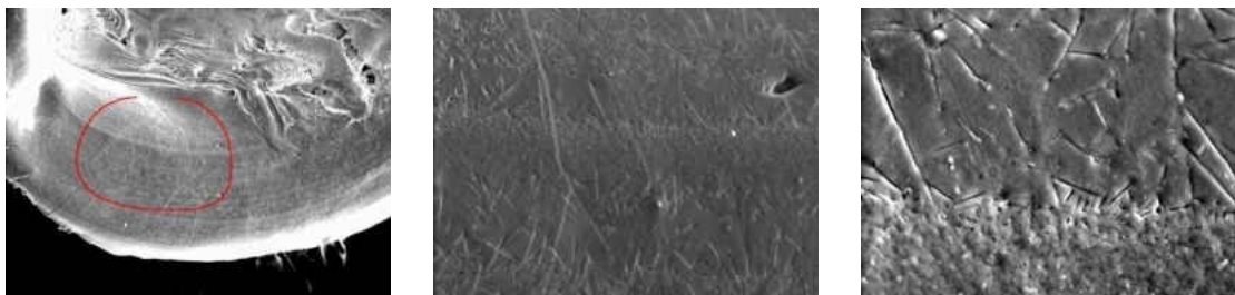
Figure 19. Surface Characteristics of 400,000 - 500,000 g/mol poly(DADMAI) at 35x, 300x, 1000x
