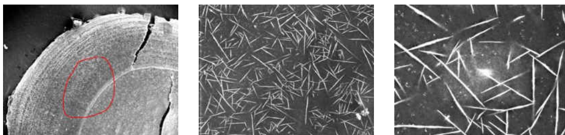
Figure 16. Surface Characteristics of <100,000 g/mol poly(DADMAC) at 35x, 300x, 1000x
