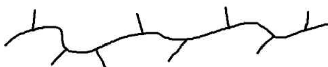
Figure 2.9. The molecular structure of LLDPE with short branches.
