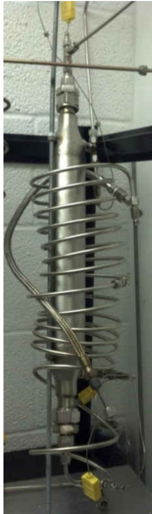
Figure 13. Double-Pipe VAM Reactor Bed
