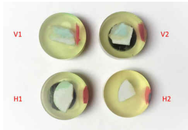
Figure 7.2 Figure 2. 3D printed rock fragments for nanoindentation experiments. 'V' represents vertical, and 'H' denotes horizontal.
