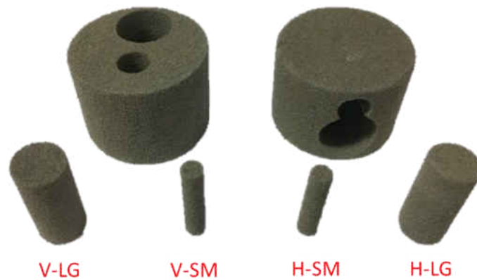
Figure 5.1 3D-printed silica sand samples and cored cylindrical plugs in vertical and horizontal directions.
