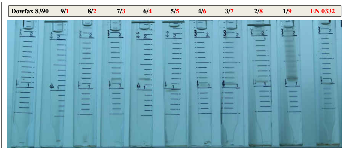
Figure 54- Blend Scan: 2% over all [Dowfax 8390&EN 0332] WOR ~1 n-Octane/Bakken Brine (309K ppm) ~105°C
