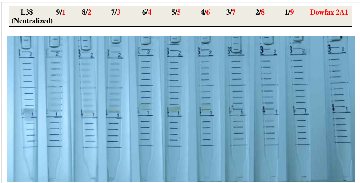
Figure 52- Blend Scan: 2% over all [L 38&Dowfax 2A1] WOR ~1 n-Octane/Bakken Brine (309K ppm) ~105°C
