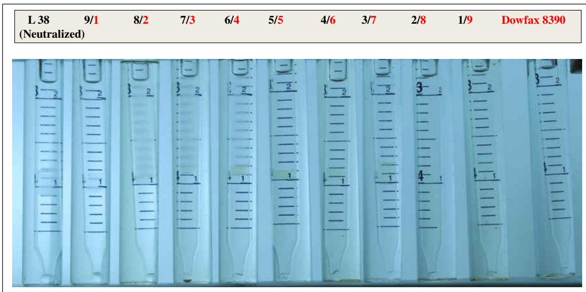
Figure 53- Blend Scan: 2% over all [L 38&Dowfax 8390] WOR ~1 n-Octane/Bakken Brine (309K ppm) ~105°C
