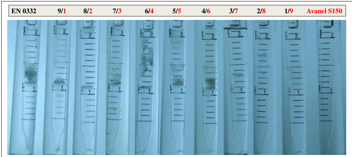
Figure 56- Blend Scan: 2% over all [EN 0332& Avel S150] WOR ~1 n-Octane/Bakken Brine (309K ppm) ~105°C
