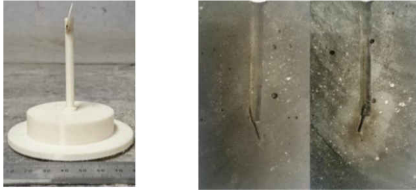
Figure 2.10: Prototype mould of the 75° pre-existing circular notch (left) and prototype specimen cut in half along the axis of the borehole, the 75° pre-existing circular notch appears at the bottom of the borehole section (Schwartzkopff, 2017).
