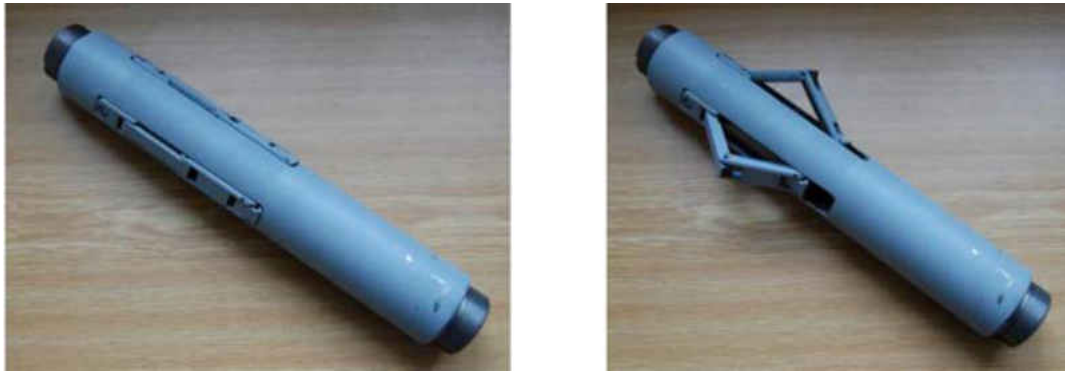
Figure 2.18: The designed indenter to create fracture in a desired direction: in transportation mode (left) and in operation (right) (Patutin and Serdyukov 2017).
