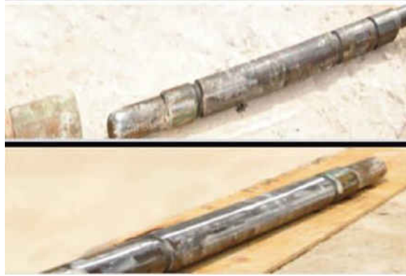
Figure 2.21: The jetting tool proposed by Abbas et al (2009) to create a vertical hole to facilitate fracture initiation.
