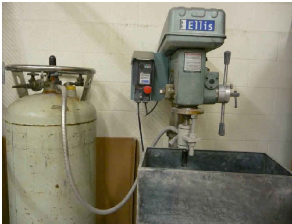
Figure 3.2 Core plug sampling system used in this study
