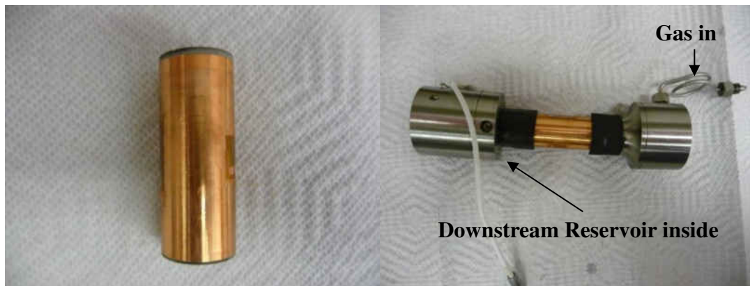
Figure 3.8 Core covered with copper sheeting, and assembled on End Caps for a low permeability test system
