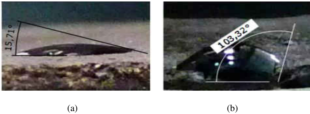
Figure 3-3 Contact angles of oil/air/rock systems treated by 100 mg/L \text{Al}_2\text{O}_3 NPs. (a) Before treatment, (b) After treatment (Giraldo et al., 2013).
