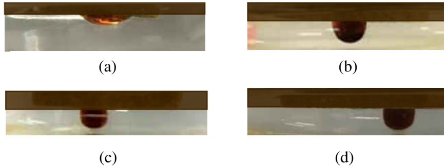
Figure 4-13 Oil contact angle. (a) 2000 mg/L KCl brine. (b) 1000 mg/L MERPOL HCS surfactant. (c) 1000 mg/L MERPOL HCS surfactant + 2000 mg/L LUDOX SM-30 nanoparticle. (d) 1000 mg/L MERPOL HCS surfactant + 2000 mg/L LUDOX TM-50 nanoparticle.
