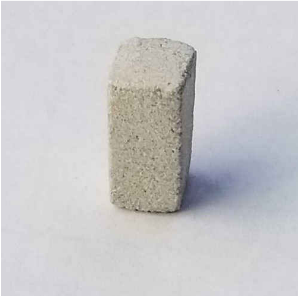
Figure 11. Core sample prepared for CT scan
