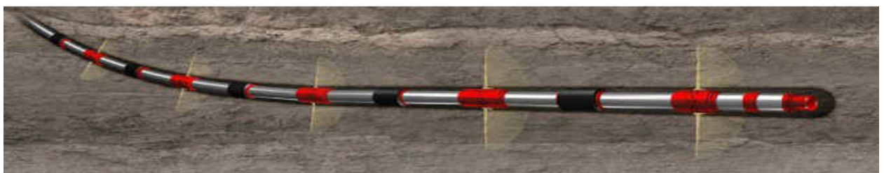
Figure 7. Multi-stage hydraulic fracturing (Rafie et al., 2014)
