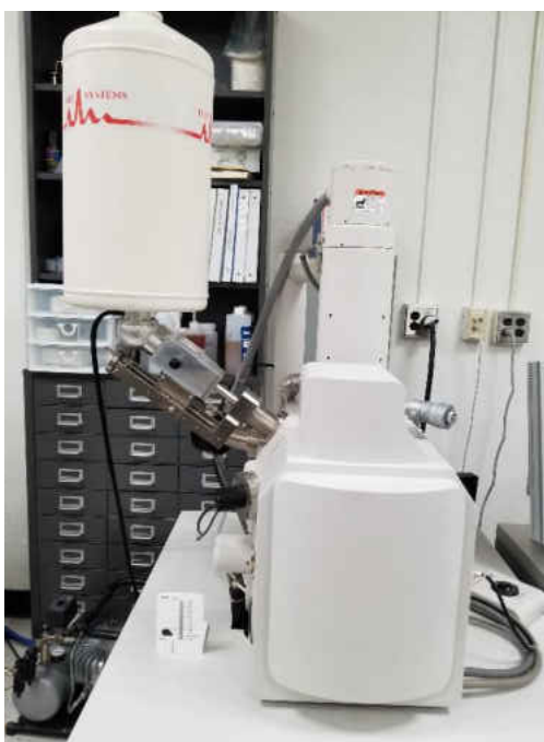
Figure 6. Hitachi S-3400NH scanning electron microscope
