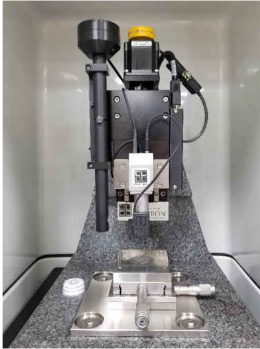
Figure 12. Hysitron TI-700 ubi nano-mechanical indenter
