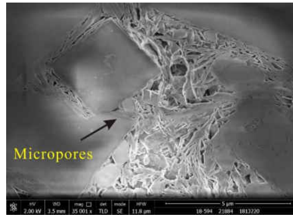
(b) Interlamellar micropores well developed in clay minerals
