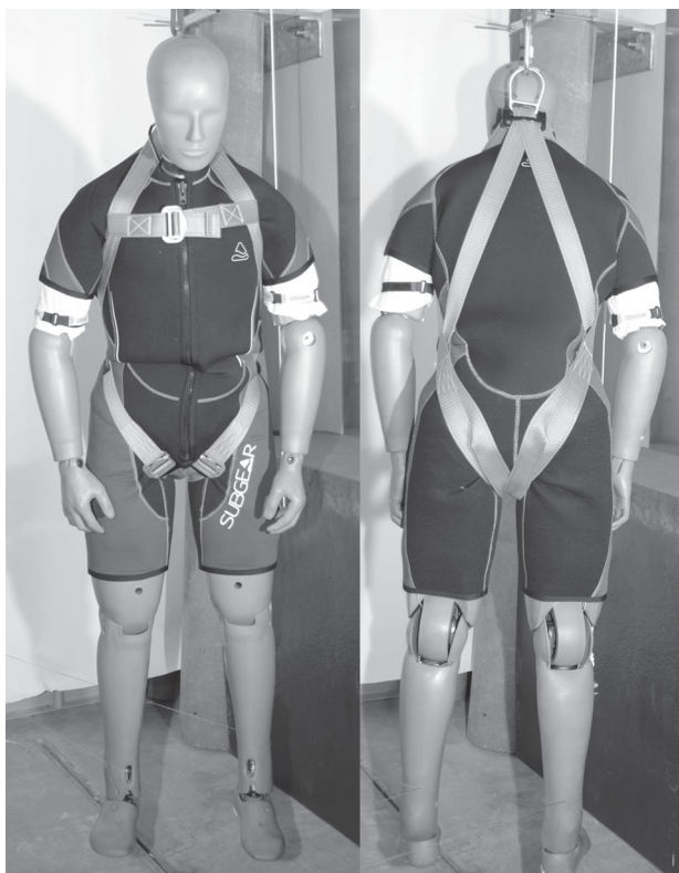
Figure 4. Position of the shoulder straps and the dorsal attachment point in a safety harness after fall arrest.
