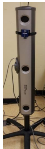
Figure 7: Optotrak Position Sensor from the three dimensional Motion Capture System
