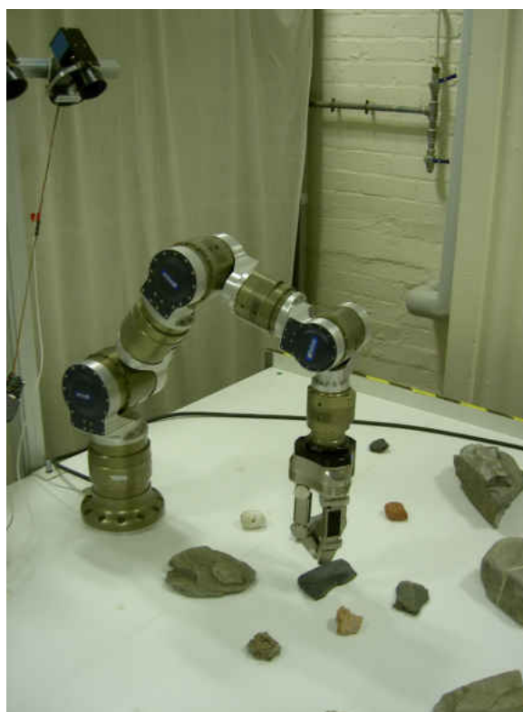
Figure 6.10: Robotic arm controlled to reach the rock which has highest science value
