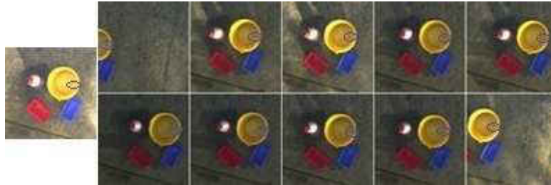
Figure 6.48 - (Stabilisation using 3.5mm lens). Blue circle indicator presents the common region across the sequence
