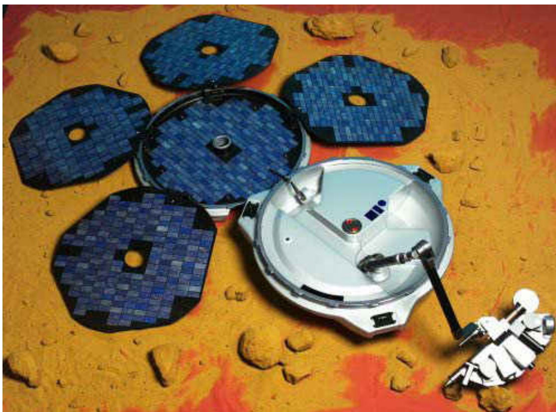
Figure 1.1: The Beagle 2 lander. The ARM would position the PAW whose calibration undertaken by Aberystwyth University to conduct panoramic, macroscopic and microscopic imaging, in-situ compositional analysis, and sample acquisition for the Gas Analysis Package (GAP) experiment (Barnes et al. , 2003; Barnes et al. , 2006). Image courtesy of ESA
