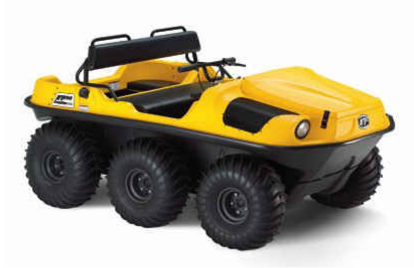
Figure 1.1: The ARGO 6x6 Frontier Amphibious Skid-Steer Off-Road Vehicle
