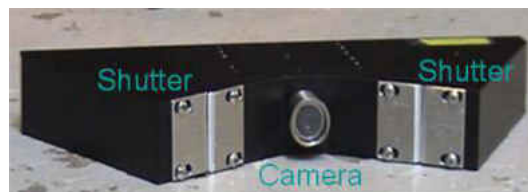
Figure 7.34: The final design of the dual laser scanner
