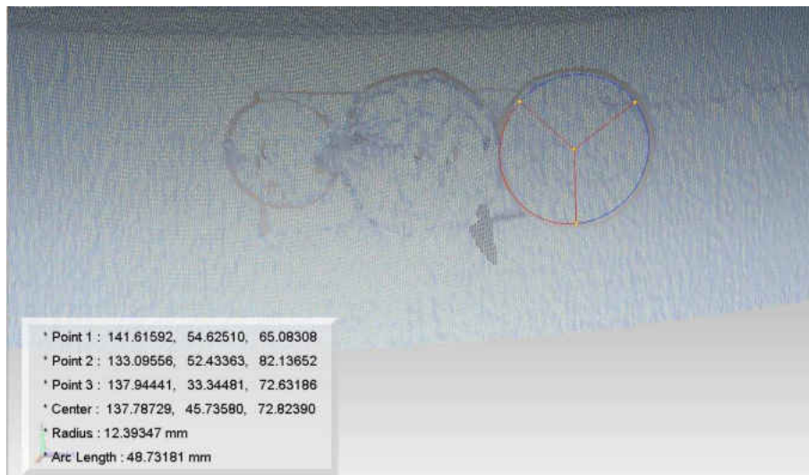
Figure 7.11: The measurement of the coins in the 3D model of the well head
