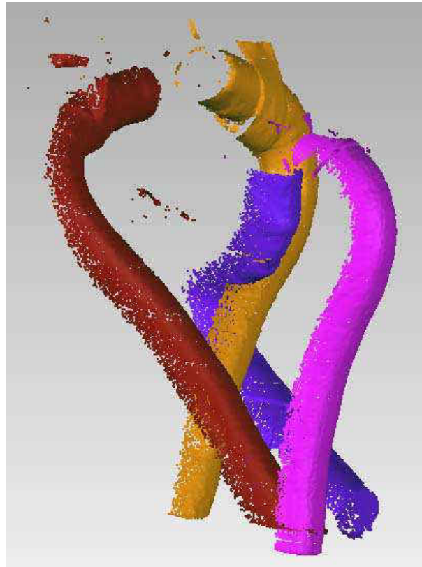
Figure 7.7: Four different 3D views of the mooring chain links from the right laser scanner
