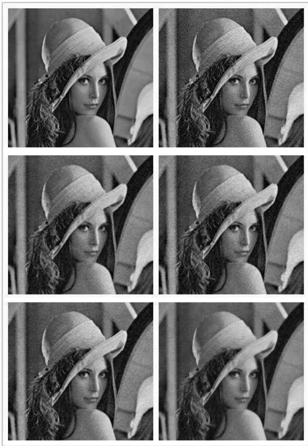
Figure 6.3: Result of denoising 'Lena' with different methods when the noise level is \sigma = 0.3 . The Sparse Code Shrinkage method was applied using the estimated orthogonalized ICA transform ( 8 \times 8 windows), while Gaussian smoothing with 3 \times 3 masks, median and wiener filtering in 3 \times 3 neighborhood. Top left: original image, top right: noise added, second row left: Gaussian smoothed, second row right: median filtered, third row left: wiener filtered, third row right: SCS applied.
