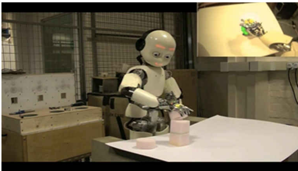
Figure 5.15: The iCub, having successfully grasped an object placed in front of it.
