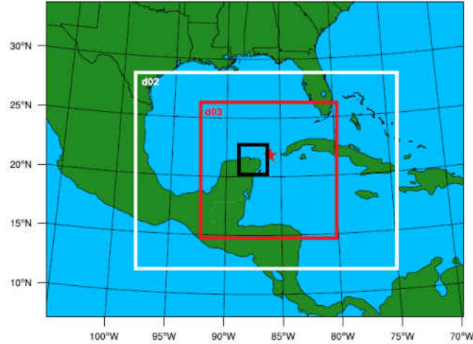
Figure 41: Model domain for 20 June 2017 simulation. D02 represents the first nest within the domain with horizontal grid spacing of 9 km and D03 represents the innermost nest of the model set up with horizontal grid spacing of 3 km (red box). Area designated for convective development analysis is represented by the black box. The red star represents the location of the aircraft at 1651 UTC.
