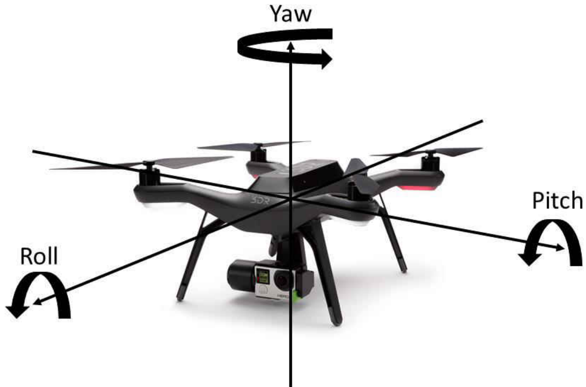
Fig. 2: Yaw, pitch, and roll with respect to a sUAS.
