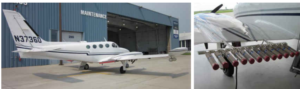
Figure 5: Image showing the Cessna 340 aircraft used during POLCAST2 and the end of POLCAST3 located at the Fargo Jet Center in Fargo, North Dakota. Shown on the right is an image of one wing with a full set of hygroscopic flares. Both images were taken during POLCAST3.
