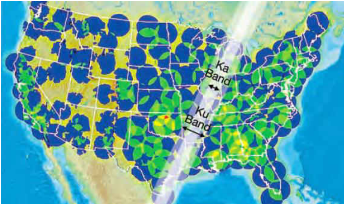
Figure. 11. Ground Radar Coverage with GPM Scan. Ground radar coverage in the contiguous United States. Overlap of radars is shaded in green, yellow, and red. An example orbit showing DPR coverage that would fill in gaps of ground radar coverage (Image from Hanson and Gray 2012).
