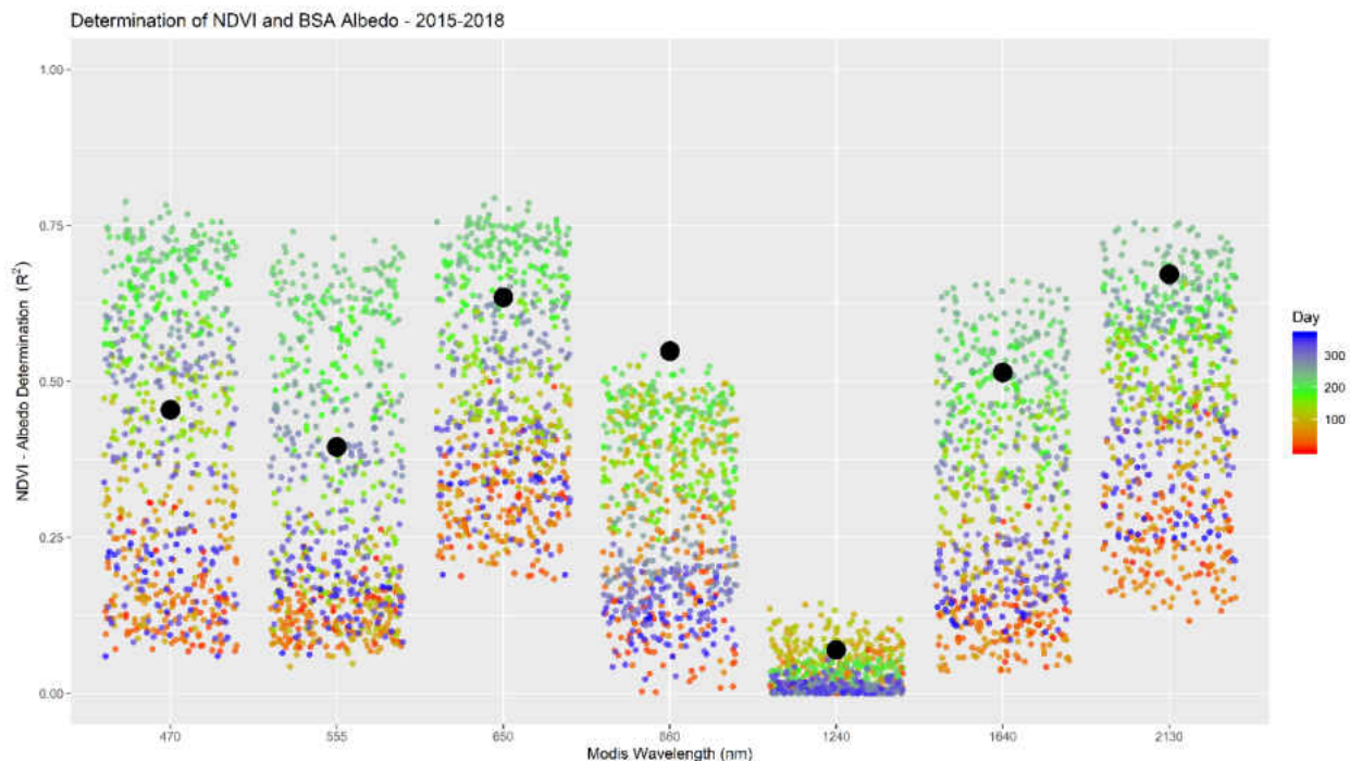
Figure 22: Coefficient of determination for each wavelength’s albedo using NDVI over United States cropland areas for 2015-2018 by day of year (colored dots) and annual total (black dots).
