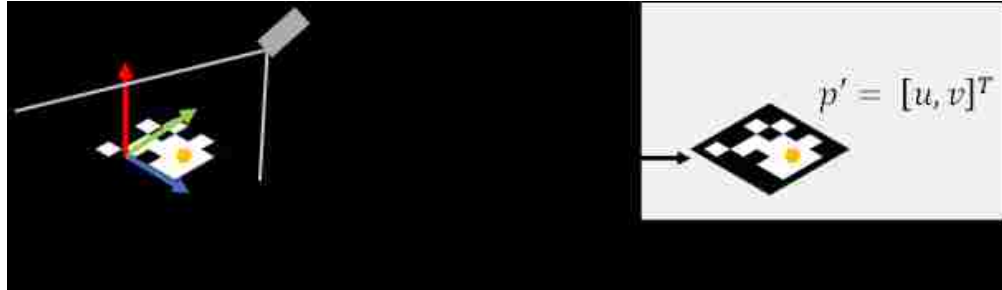
Figure 2.5. The homography transformation between the two coordinate systems
