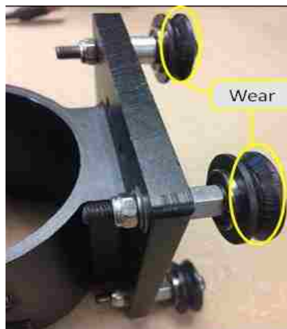
Figure 4.12. The wear of a V-wheel mechanism caused by the installation error
