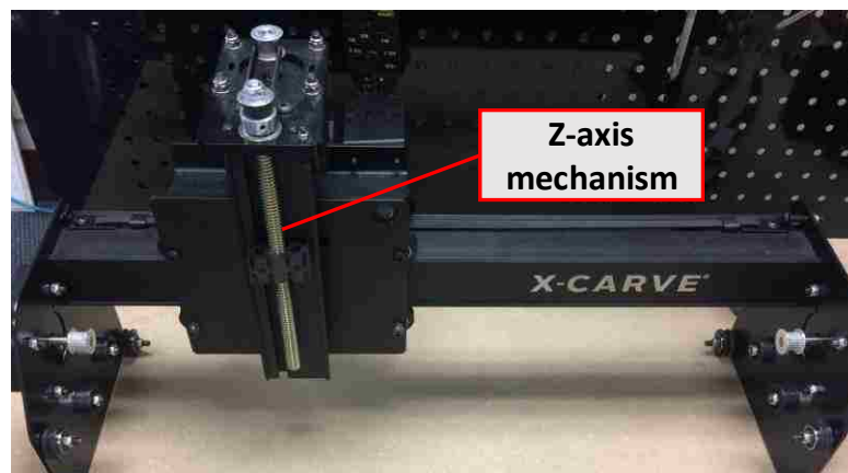
Figure 3.2. The z-axis mechanism of the spindle assembly
