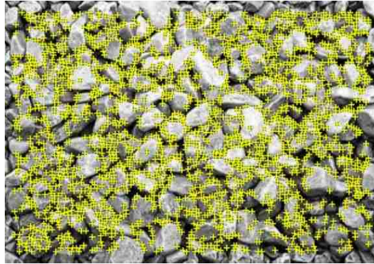
Figure 2.3. The detected features (corners) on the marker. Corners represent the regions which have the highest change in intensity in all directions, which are highlighted with yellow '+'.
