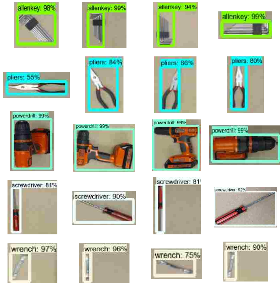
Figure 4.4. The results of detecting real tools with various orientations
