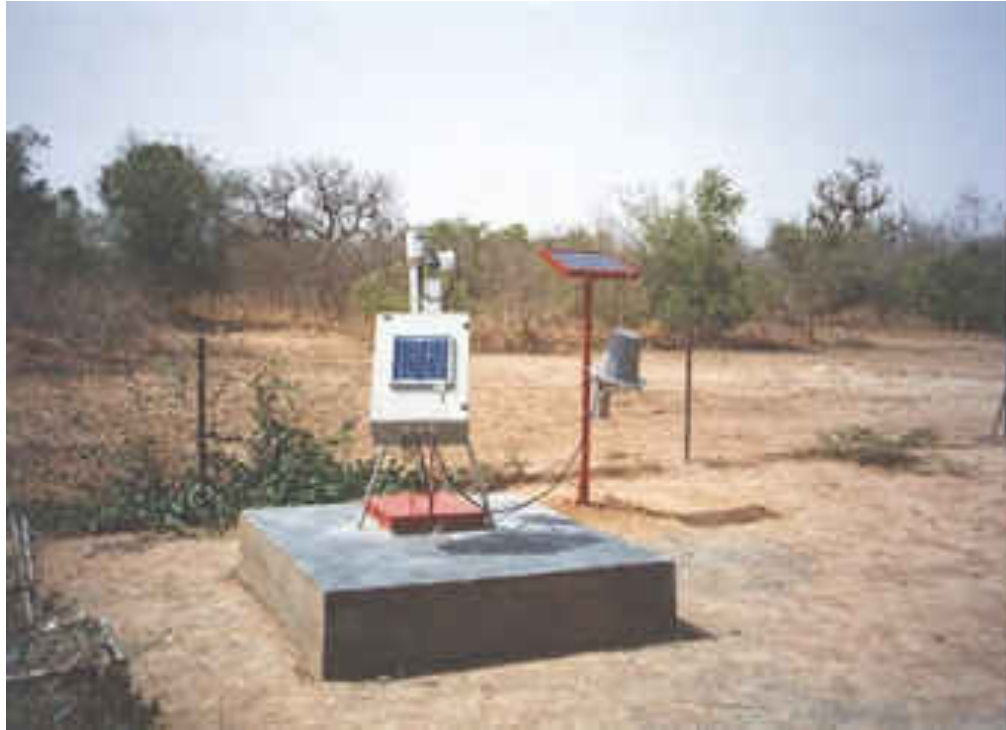
Figure 4. The AERONET instrument at the IER Cinzana site in rural Mali, West Africa is located on a concrete platform in a cultivated region.
