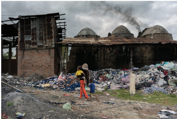
Figure 1. A mother and her children walk past a burning brick kiln fuelled by garment off-cuts (Photo by Thomas Cristofolletti; copyright Royal Holloway University of London [RHUL]).
