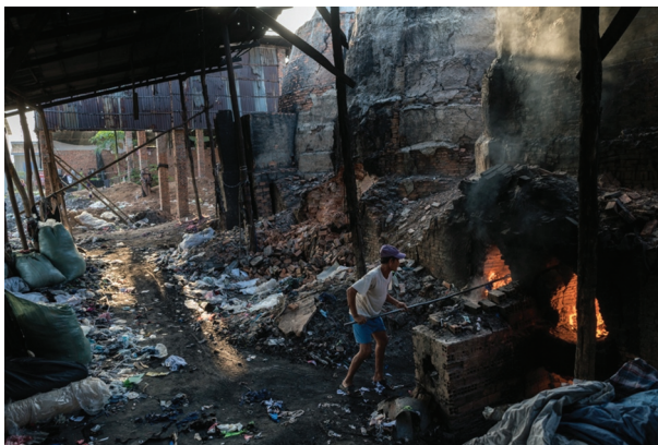
Figure 4. A brick worker stokes the kiln fire with garment waste (Photo by Thomas Cristofolletti; copyright RHUL).
