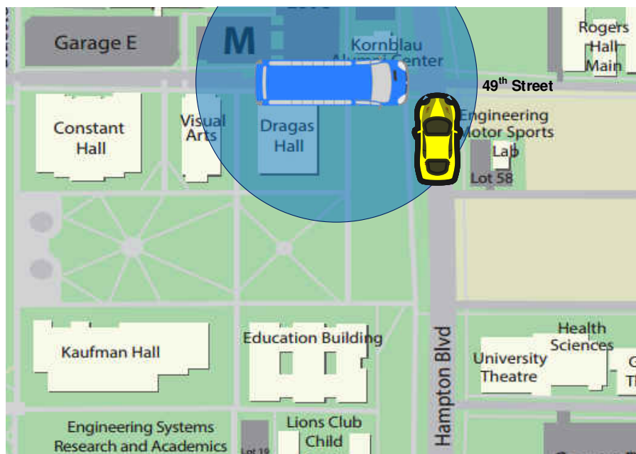
FIG. 21: Misleading vehicle location and direction provided by a mobile BlueCollect unit
