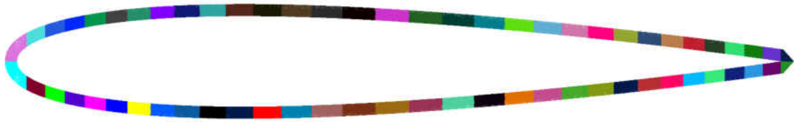
Fig. 21. Decomposed Delaunay subdomains for NACA 0012 Airfoil
