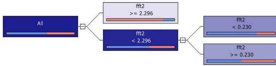
FIG. 4.4: Excel SQL Datamining tool Feature Extraction (Decision Tree Algorithm). The blue part in the first box represents the cars. It shows that around 60% of the cars have the value fft2 less than 2.296
