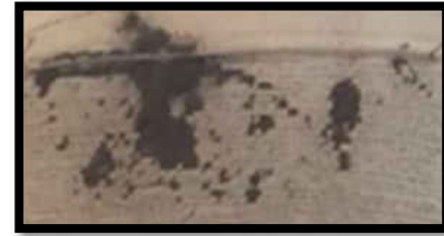
Figure 9.3-8. 10-50 \mu\text{m} dust dropped over the knee. Clusters of dust covered a small section of the fabric
