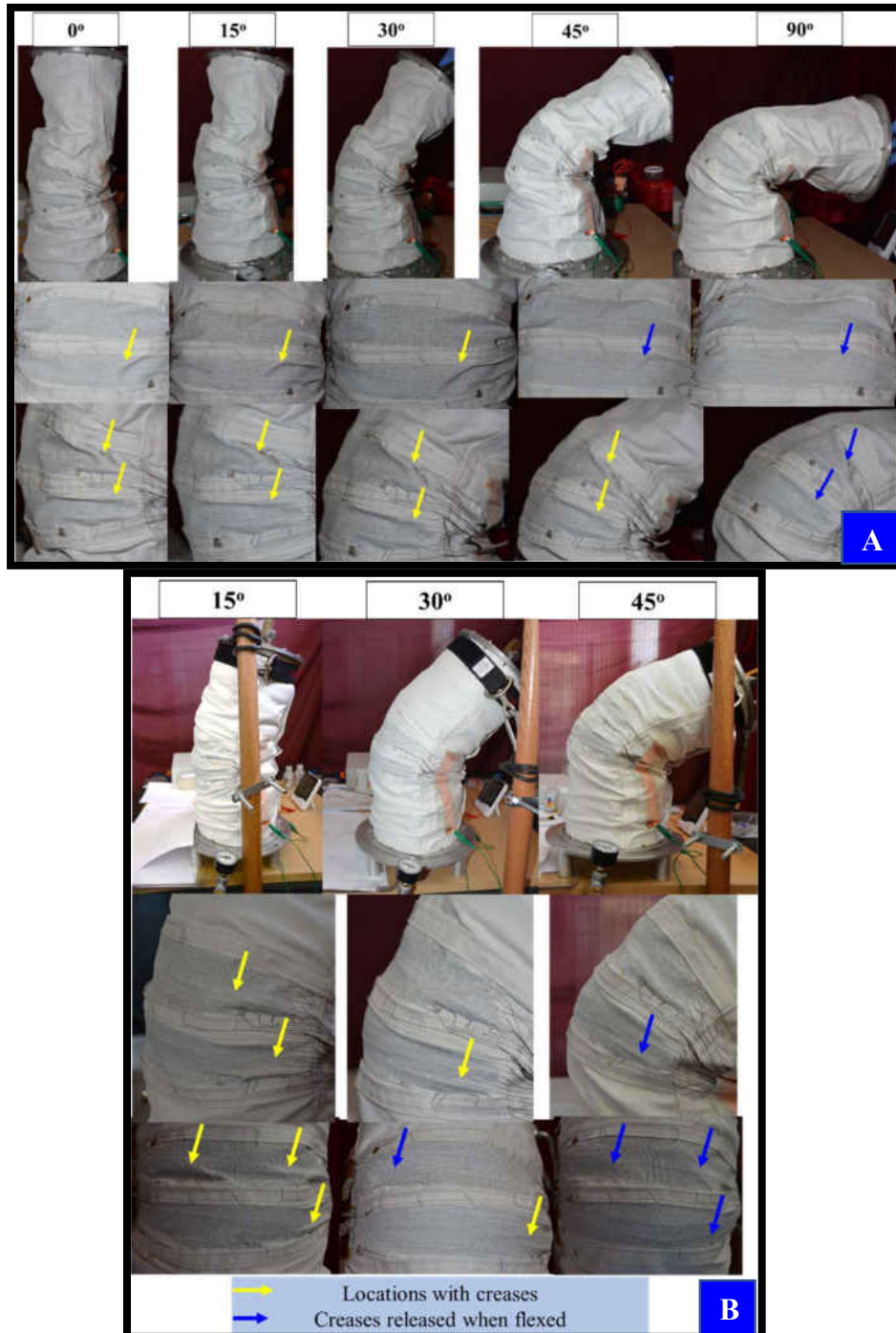
Figure 9.3-1. [A] Unpressurized and [B] Pressurized module. Arrows point to creases in the knee area
