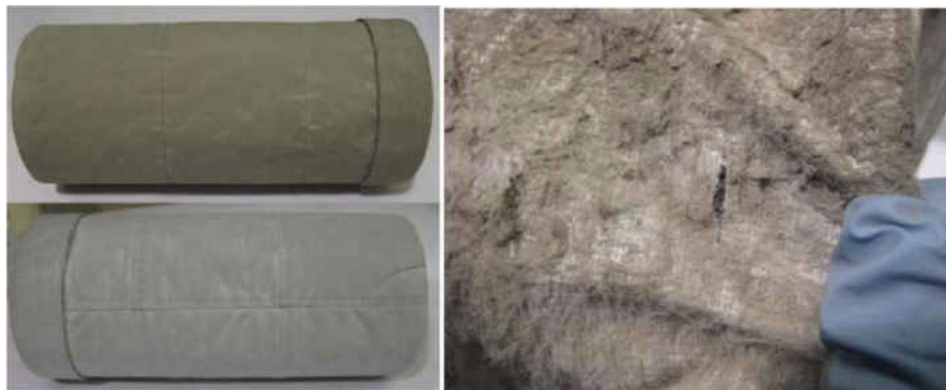
Figure 2.7-3. [Left] Comparison of hue between simulant types. Top picture using JSC-1 simulant and bottom using NU-LHT-2C, both using W.L. Gore 4 fabric. [Right] Close-up of damaged Tyvek fabric with a tear (Mitchell ,2010)
