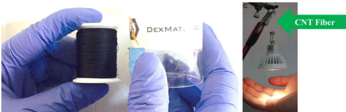
Figure 4.3-1. [Left] DexMat’s CNT fibers utilized in current research experiments, [Right] Display of strength and utilization of CNT fiber developed by Rice University. Suspending a 46g light-emitting diode lit using two 24- \mu m-thick CNT fibers (Behabtu et al., 2013)
