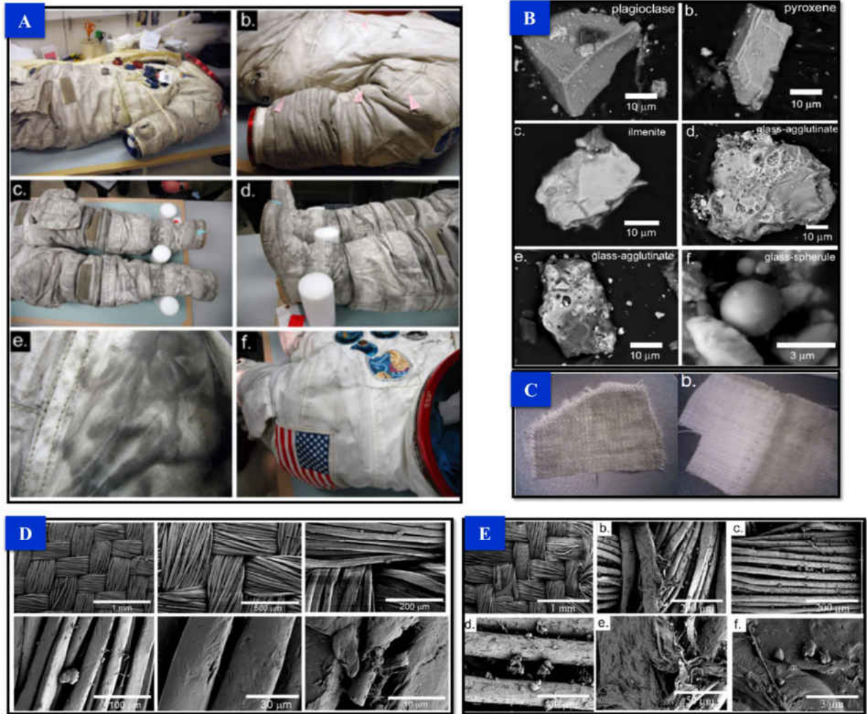
Figure 2.5-4. [A] Apollo 17 A7LB spacesuit during post flight investigations, [B] SEM images of particles from the surface of the Apollo 17 T-164 Teflon outerfabric, [C] Samples of outer fabric from Apollo 12 spacesuit, left is from left knee and right side is from left shoulder where the lighter area was covered under U.S. flag patch, [D] SEM secondary electron images of T-164 Teflon from left knee area of Apollo 12, [E] T-164 Teflon fabric from unexposed area on left shoulder on Apollo 12 ITMG covered by the flag patch ( All pictures from Christoffersen et al., study in 2008 ).
