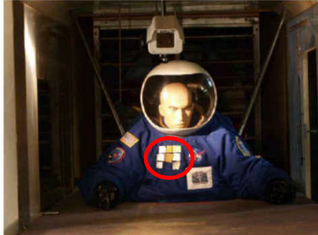
Figure 2.7-4. NDX-1 spacesuit in the test position in MARSWIT. The 9 sample patches are seen on the right of the mannequin (Gaier et al., 2010)
