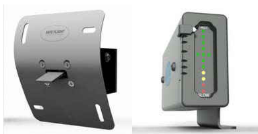
Figure 15. Safe Flight SCx Lift Transducer and Indexer Computer (Safe Flight, News Release, 2014)
