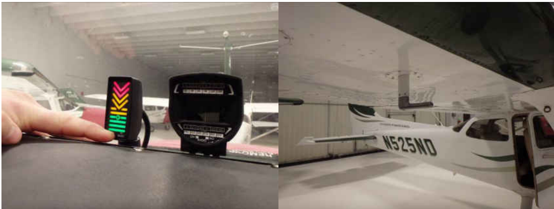
Figure 18. Garmin GI 260 Installation on N525ND
