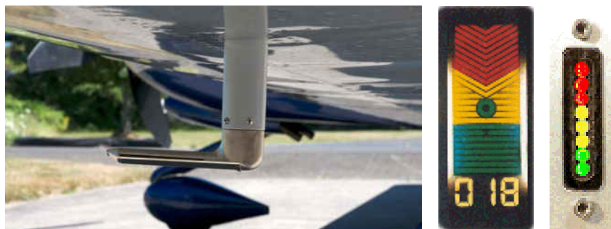
Figure 5. left to right: Advanced Flight Systems AOA probe, Pro III, and Sport (Advanced Flight Systems, 2014)
